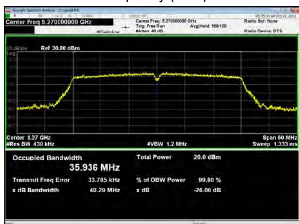
U-NII-2A, 802.11ac VHT40 Carrier frequency (MHz): 5270
