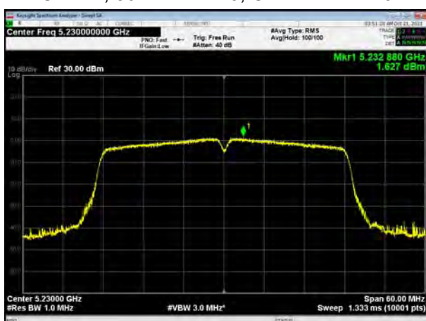
U-NII-1, 802.11ac VHT40, Channel No.: 38
