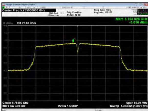
U-NII-3, 802.11ac VHT40, Channel No.: 151
