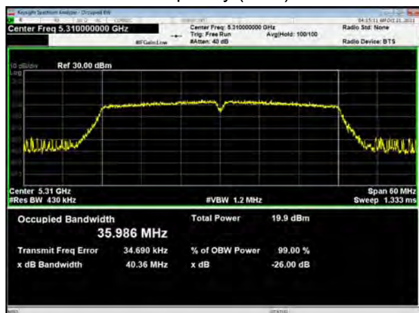
U-NII-2A, 802.11ac VHT40 Carrier frequency (MHz): 5270
