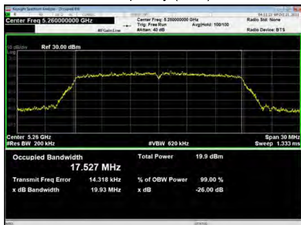
U-NII-2A, 802.11ac VHT20 Carrier frequency (MHz): 5300
