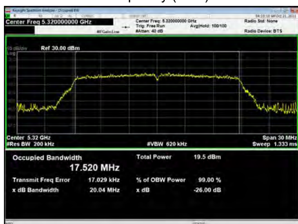
U-NII-2A, 802.11n HT20 Carrier frequency (MHz): 5320
