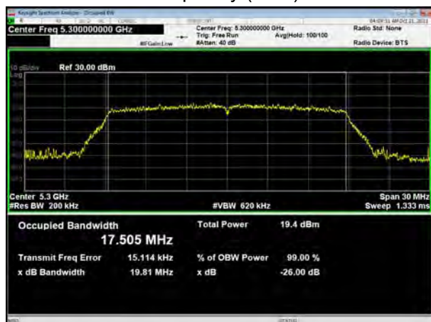
U-NII-2A, 802.11n HT20 Carrier frequency (MHz): 5320
