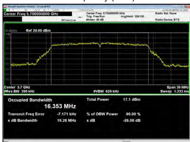
U-NII-2C, 802.11a Carrier frequency (MHz): 5700
