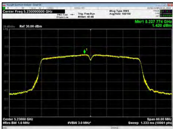
U-NII-1, 802.11ac VHT40, Channel No.: 46
