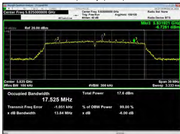
U-NII-3, 802.11ac VHT20 Carrier frequency (MHz): 5745
