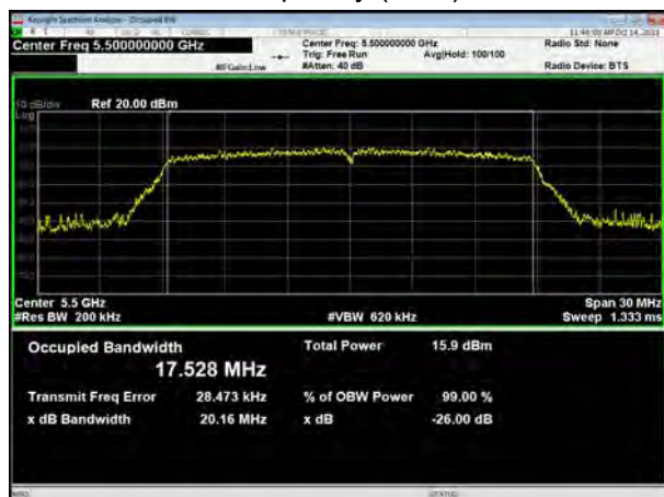
U-NII-2C, 802.11n HT20 Carrier frequency (MHz): 5580
