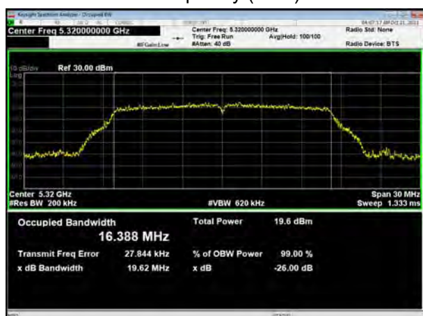
U-NII-2A, 802.11a Carrier frequency (MHz): 5320
