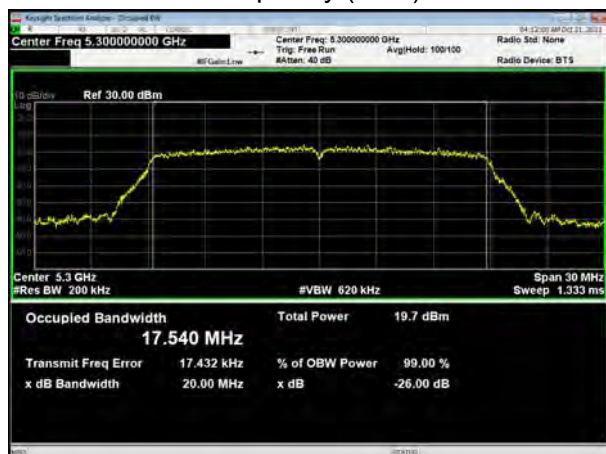
U-NII-2A, 802.11ac VHT20 Carrier frequency (MHz): 5320
