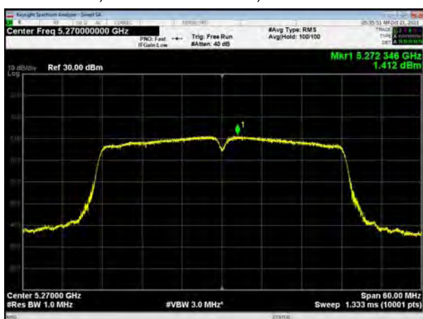
U-NII-2A, 802.11ac VHT40, Channel No.: 54
