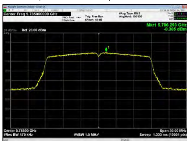
U-NII-3, 802.11ac VHT20, Channel No.: 165
