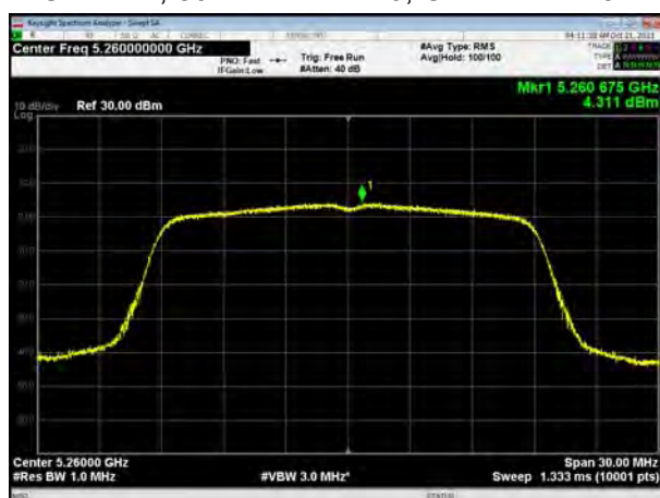
U-NII-2A, 802.11ac VHT20, Channel No.: 60
