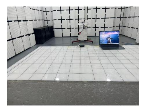
Set-up for Radiated Spurious Emission, Above 1GHz
