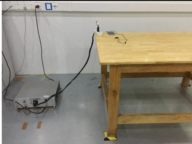
Conducted Emissions Test Setup Front View
