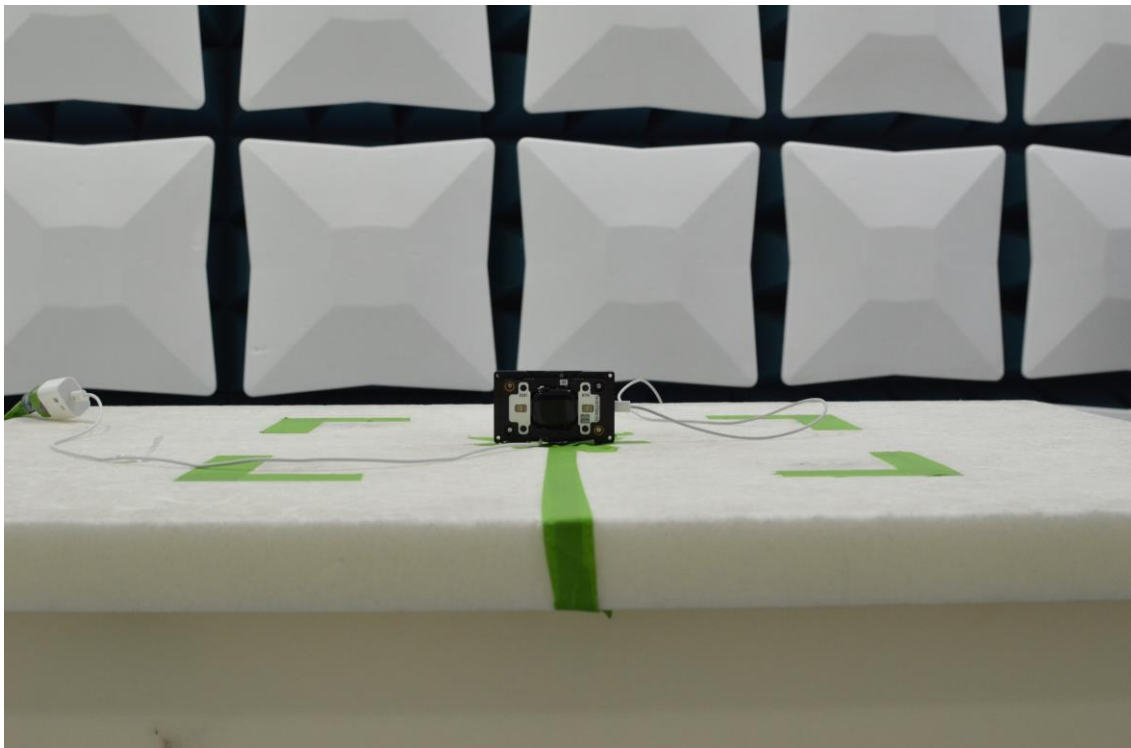
Figure 8: 1-18GHz Test Setup (Front View)
