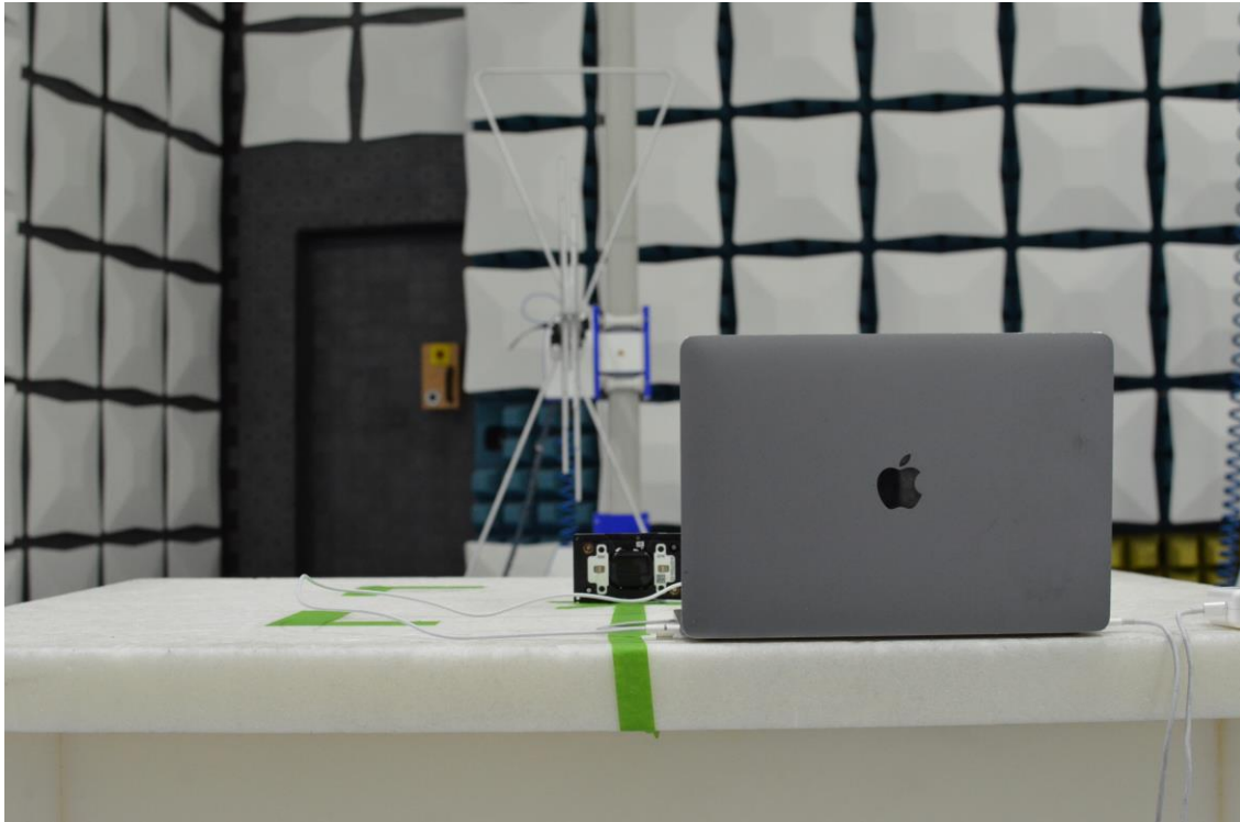
Figure 15: 30MHz-1GHz Test Setup (Rear View)
