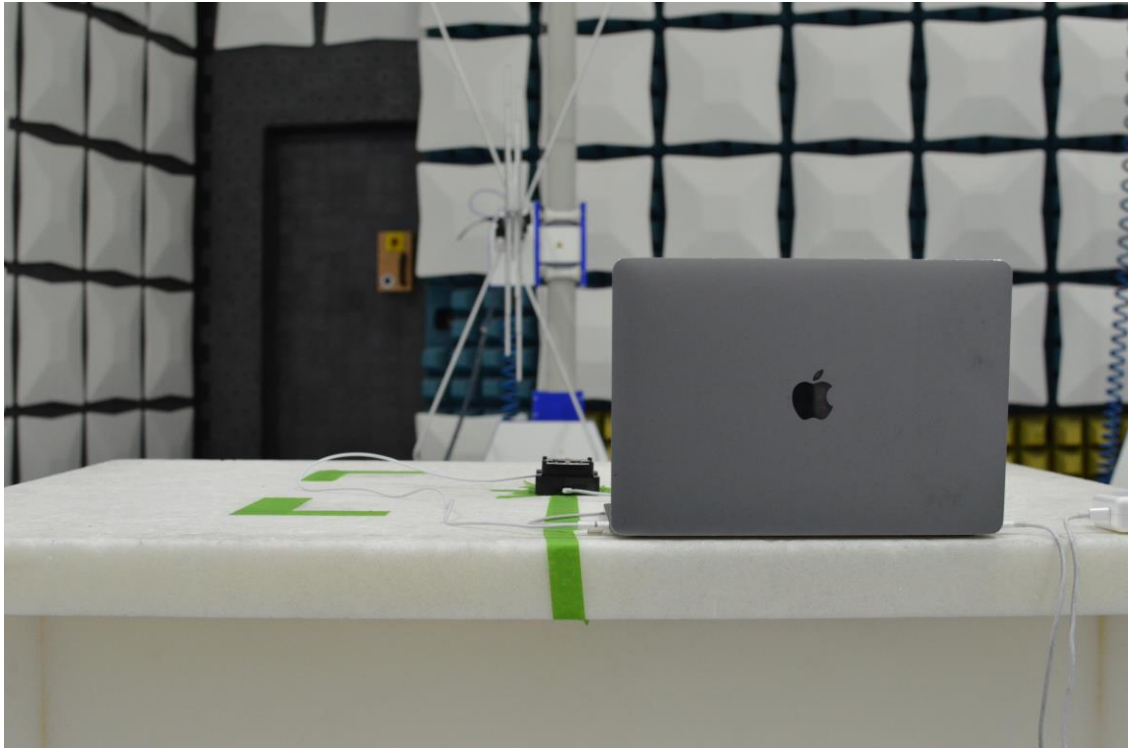
Figure 13: 30MHz-1GHz Test Setup (Rear View)
