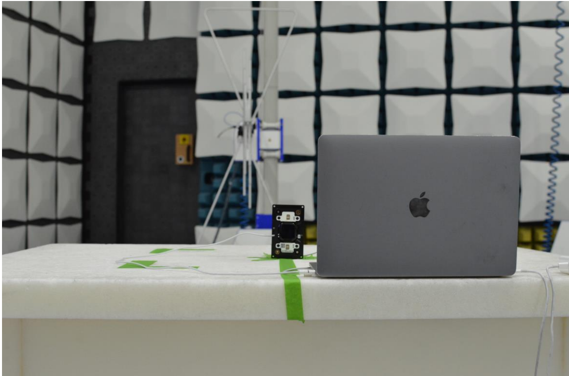
Figure 17: 30MHz-1GHz Test Setup (Rear View)
