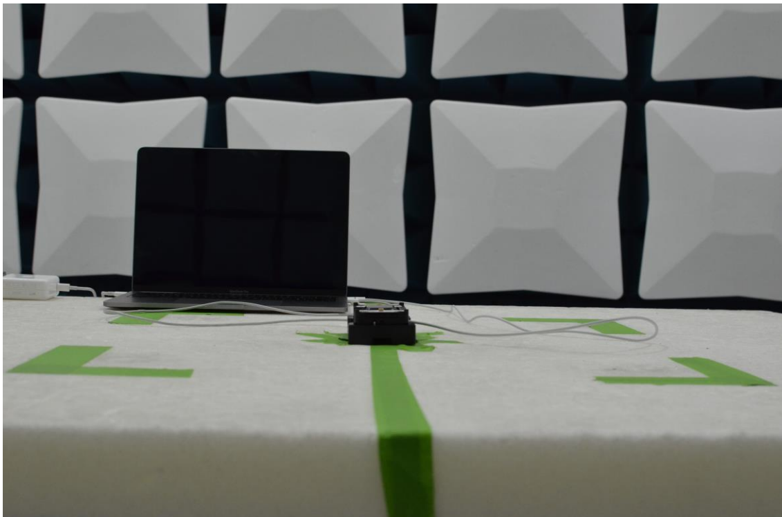
Figure 12: 30MHz-1GHz Test Setup (Front View)
