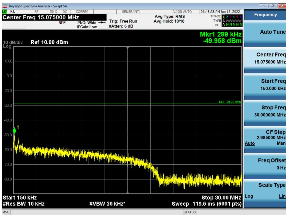
**Antenna 1 / 30 MHz ~ Low Edge - 100 MHz / B5 DSS 10 MHz 1 Carrier + 5G NR n5 10 MHz 1 Carrier [2 Carrier] / Contiguous / QPSK / Low**
