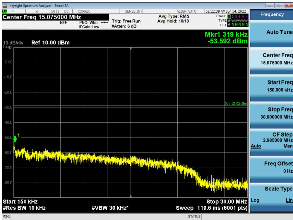
**Antenna 1 / 30 MHz ~ Low Edge - 100 MHz / B5 DSS 10 MHz 1 Carrier + 5G NR n5 10 MHz 1 Carrier + LTE B5 5 MHz 1 Carrier [3 Carrier] / Contiguous / 64QAM / Middle**
