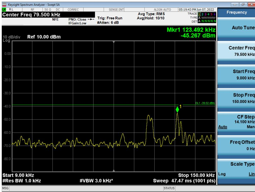
**Antenna 1 / 150 kHz ~ 30 MHz / 5G NR n5 10 MHz 1 Carrier + 5G NR n5 10 MHz 1 Carrier [2 Carrier] / Contiguous / 256QAM / Low**
