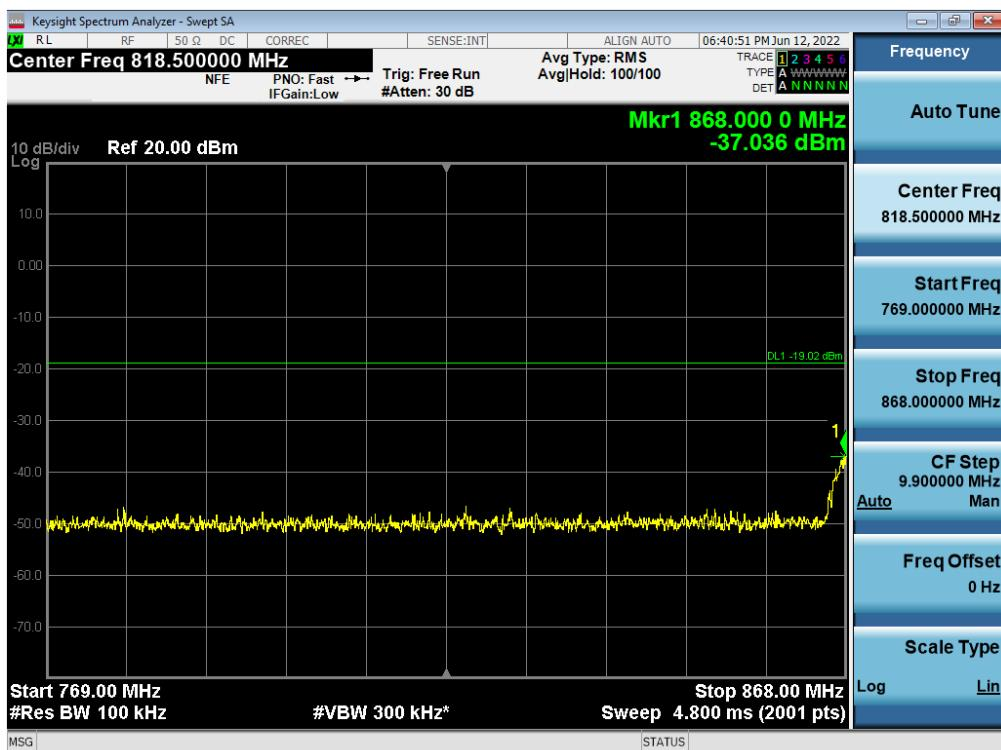
**Antenna 0 / High Edge ~ 1 GHz / 5G NR n5 10 MHz 1 Carrier + 5G NR n5 10 MHz 1 Carrier + LTE B5 5 MHz 1 Carrier [3 Carrier] / Contiguous / 64QAM / Middle**
