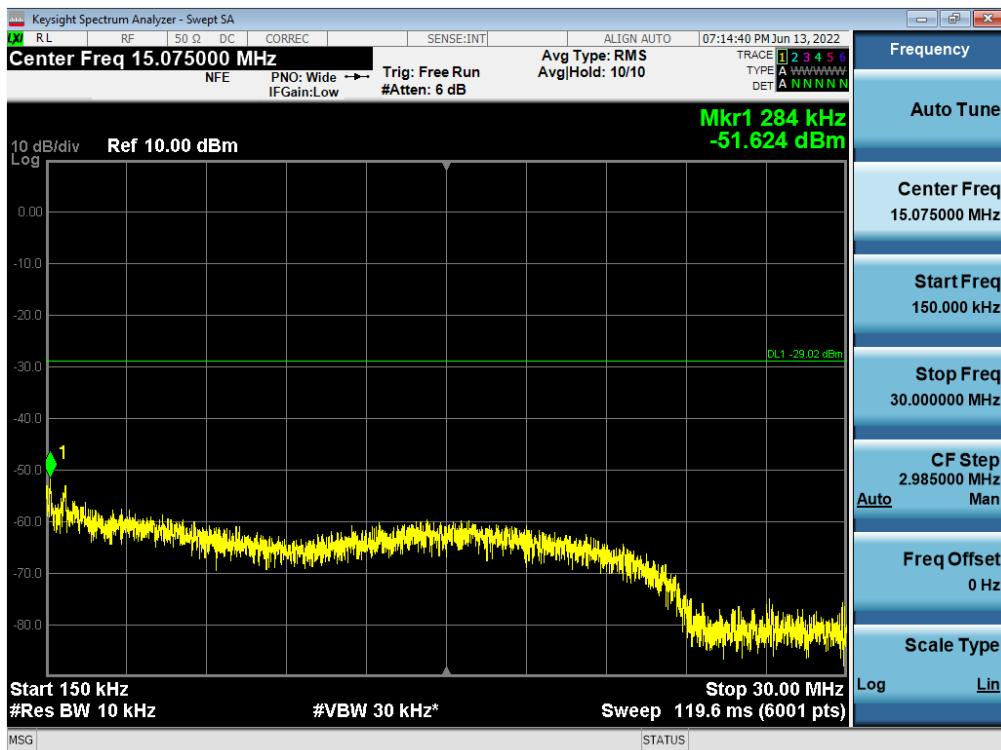
**Antenna 1 / 30 MHz ~ Low Edge - 100 MHz / B5 DSS 10 MHz 1 Carrier + 5G NR n5 10 MHz 1 Carrier [2 Carrier] / Non-Contiguous / QPSK**
