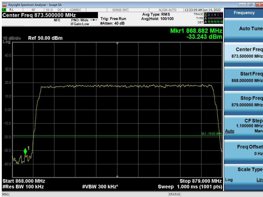
**Antenna 0 / (B5 DSS 10 MHz 1 Carrier + LTE B5 5 MHz 1 Carrier) + 5G NR n5 5 MHz 1 Carrier [3 Carrier] (2C+1C) / Non-Contiguous / QPSK / High**
