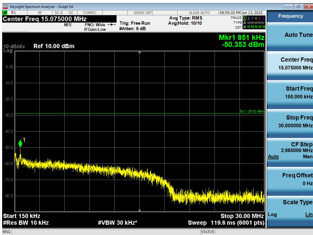
**Antenna 1 / 30 MHz ~ Low Edge - 100 MHz / B5 DSS 10 MHz 1 Carrier + 5G NR n5 5 MHz 1 Carrier + LTE B5 5 MHz 1 Carrier [3 Carrier] / Contiguous / 16QAM / Middle**
