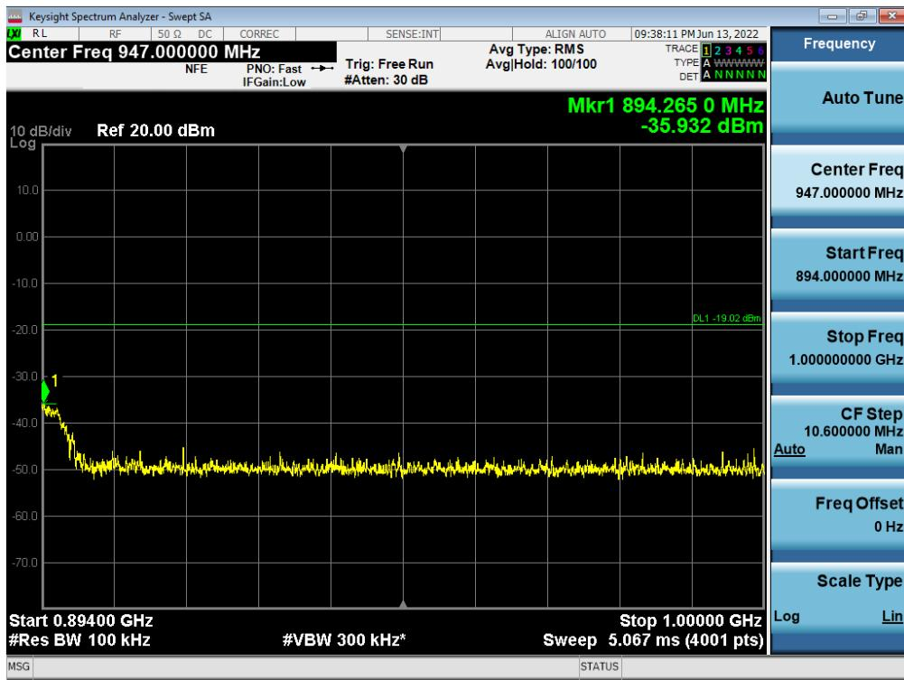
**Antenna 0 / 1 GHz ~ 10 GHz / B5 DSS 10 MHz 1 Carrier + 5G NR n5 5 MHz 1 Carrier + LTE B5 5 MHz 1 Carrier [3 Carrier] / Contiguous / 256QAM / High**
