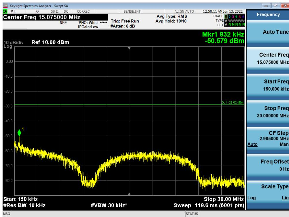
**Antenna 1 / 30 MHz ~ Low Edge - 100 MHz / B5 DSS 10 MHz 1 Carrier + 5G NR n5 5 MHz 1 Carrier [2 Carrier] / Non-Contiguous / 16QAM**
