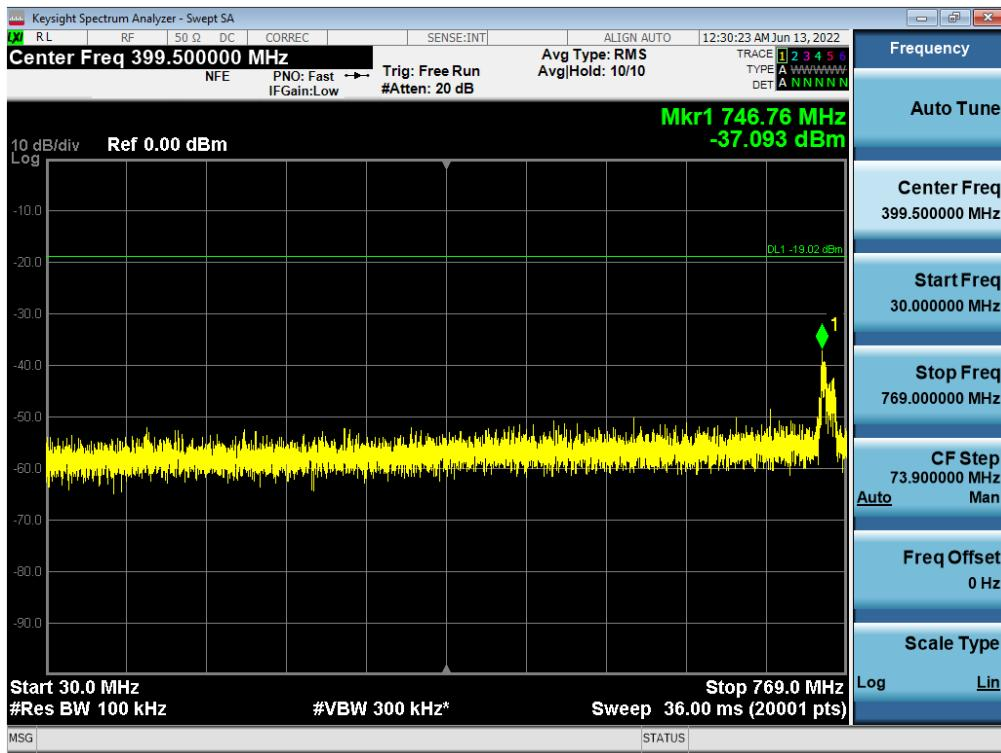
**Antenna 1 / Low Edge - 100 MHz ~ Low Edge / B5 DSS 10 MHz 1 Carrier + 5G NR n5 5 MHz 1 Carrier [2 Carrier] / Non-Contiguous / 64QAM**
