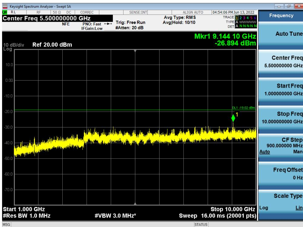
**Antenna 2 / 9 kHz ~ 150 kHz / B5 DSS 10 MHz 1 Carrier + 5G NR n5 5 MHz 1 Carrier + LTE B5 5 MHz 1 Carrier [3 Carrier] / Contiguous / 64QAM / Low**
