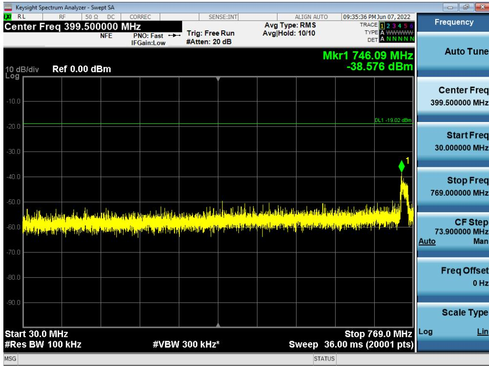
**Antenna 2 / Low Edge - 100 MHz ~ Low Edge / 5G NR n5 10 MHz 1 Carrier + 5G NR n5 10 MHz 1 Carrier [2 Carrier] / Non-Contiguous / 16QAM**
