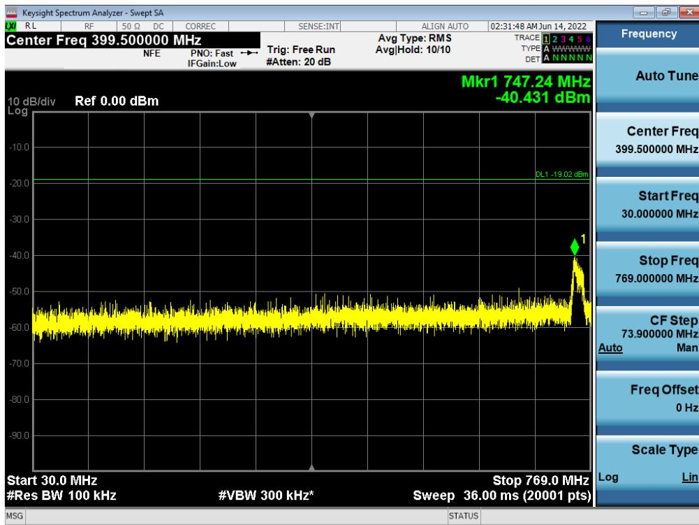
**Antenna 0 / Low Edge - 100 MHz ~ Low Edge / B5 DSS 10 MHz 1 Carrier + 5G NR n5 10 MHz 1 Carrier + LTE B5 5 MHz 1 Carrier [3 Carrier] / Contiguous / QPSK / Middle**
