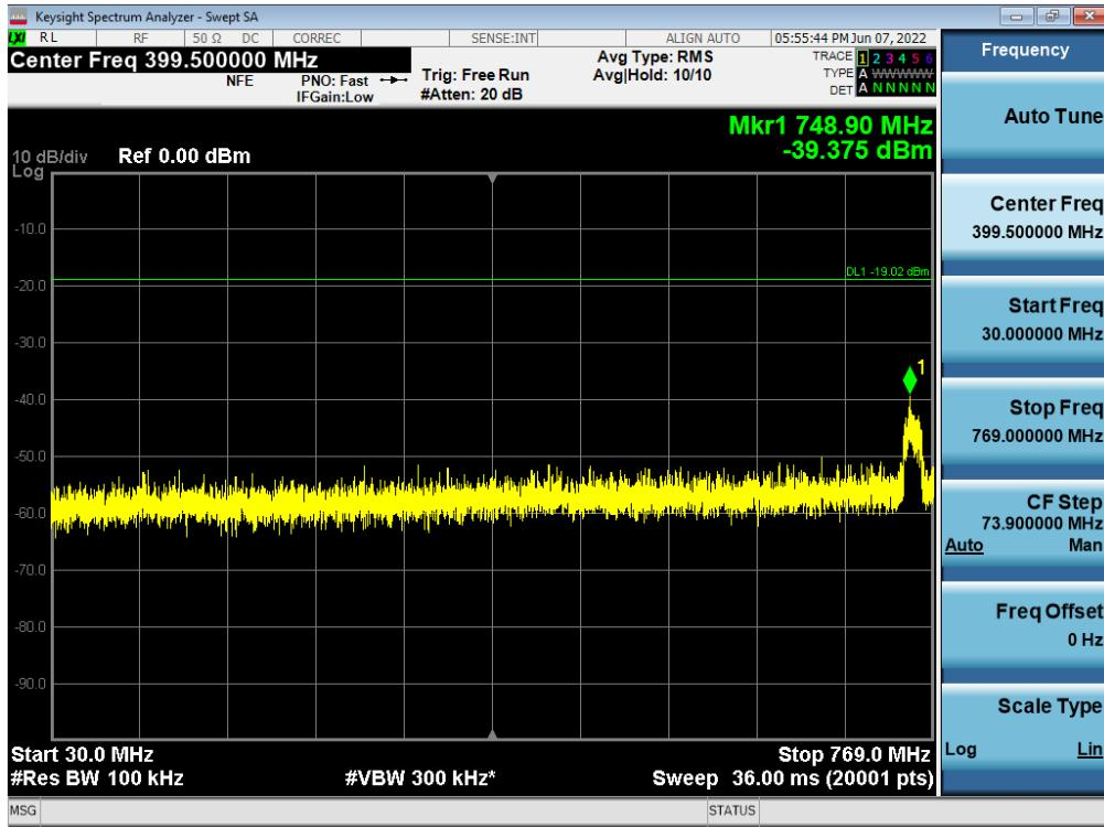
**Antenna 1 / Low Edge - 100 MHz ~ Low Edge / 5G NR n5 10 MHz 1 Carrier + 5G NR n5 10 MHz 1 Carrier [2 Carrier] / Contiguous / 256QAM / Low**
