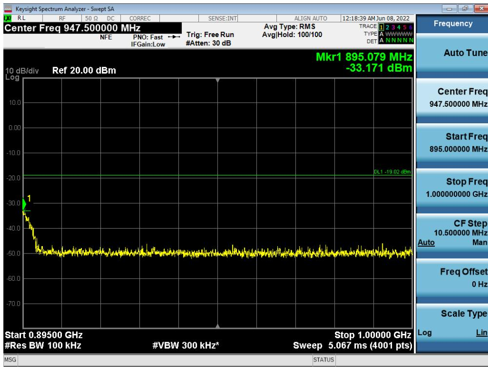
**Antenna 0 / 1 GHz ~ 10 GHz / 5G NR n5 5 MHz 1 Carrier + 5G NR n5 5 MHz 1 Carrier [2 Carrier] / Contiguous / 64QAM / Low**
