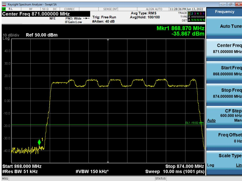
**Antenna 1 / 5G NR n5 5 MHz 1 Carrier + (LTE B5 5 MHz 1 Carrier + B5 DSS 10 MHz 1 Carrier) [3 Carrier] (1C+2C) / Non-Contiguous / 64QAM / High**
