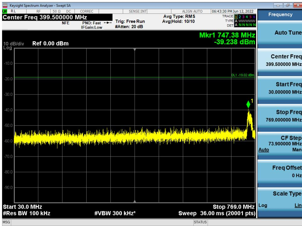
**Antenna 0 / Low Edge - 100 MHz ~ Low Edge / 5G NR n5 10 MHz 1 Carrier + 5G NR n5 10 MHz 1 Carrier + LTE B5 5 MHz 1 Carrier [3 Carrier] / Contiguous / QPSK / Middle**
