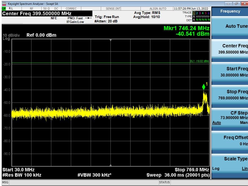
**Antenna 1 / Low Edge - 100 MHz ~ Low Edge / 5G NR n5 5 MHz 1 Carrier + (LTE B5 5 MHz 1 Carrier + B5 DSS 10 MHz 1 Carrier) [3 Carrier] (1C+2C) / Non-Contiguous / 256QAM**
