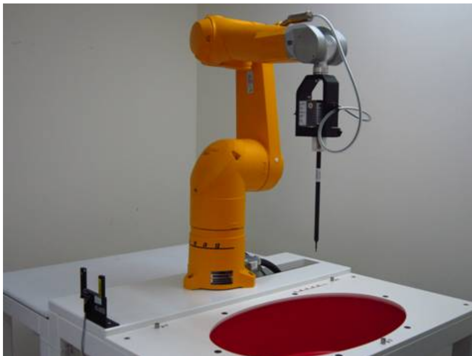
Fig.1 Photograph of the SAR measurement system
