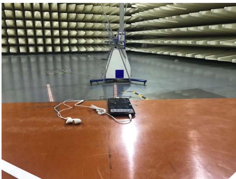
Radiated Emissions Test Setup (with charger)
