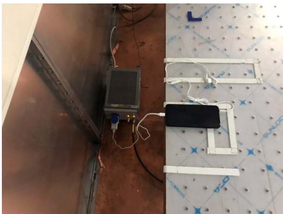
Conducted Emissions Test Setup (with charger)
