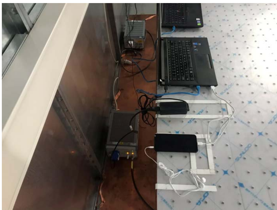
Conducted Emissions Test Setup (with laptop)
