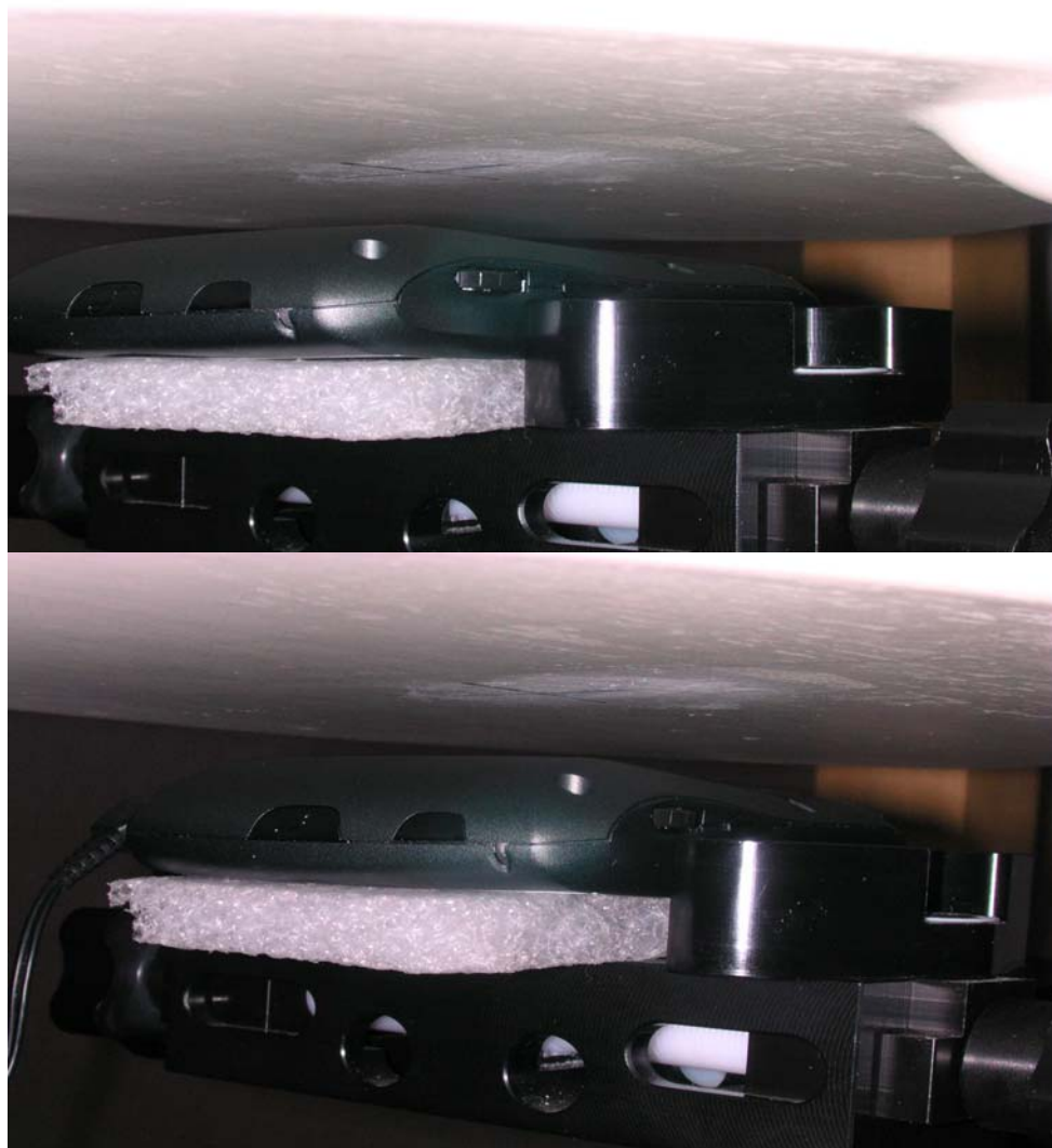
Figure 2: Photos with 15 mm separation distance
