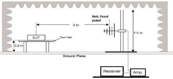
3. Radiated Emission Test-Up Frequency Above 1GHz
