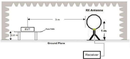
2. Radiated Emission Test-Up Frequency 30MHz~1GHz
