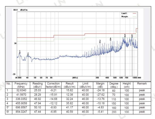
Remark: Absolute Level = Reading Level + Factor, Margin = Absolute Level – Limit Factor = Ant. Factor + Cable Loss – Pre-amplifier
