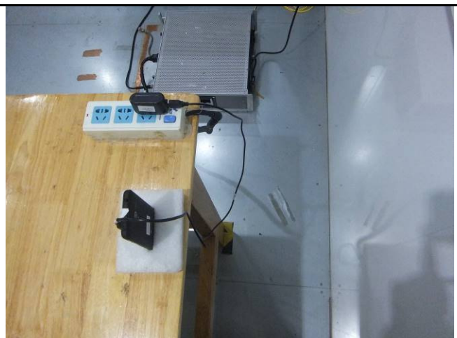
Conducted Emissions Test Setup Side View
