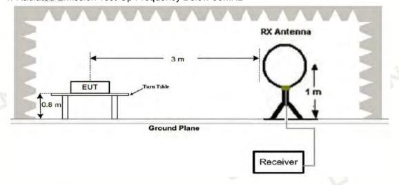
2. Radiated Emission Test-Up Frequency 30MHz~1GHz
