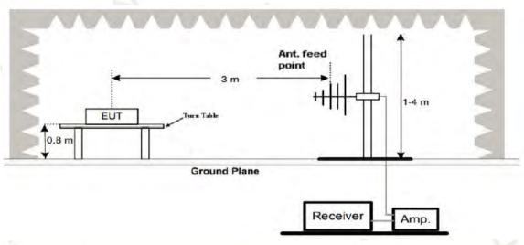
3. Radiated Emission Test-Up Frequency Above 1GHz
