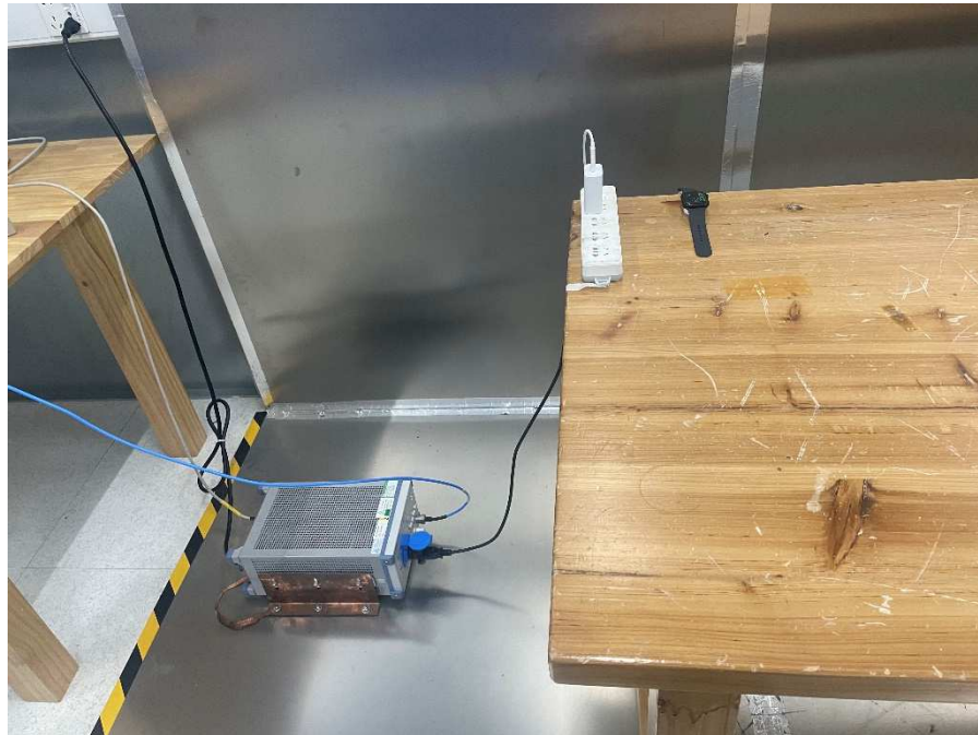
Photograph 3: Set-up photo for Conducted Emission
