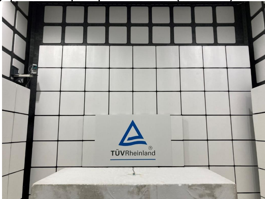
Photograph 2: Test Setup for Spurious Emissions (Front View 2)
