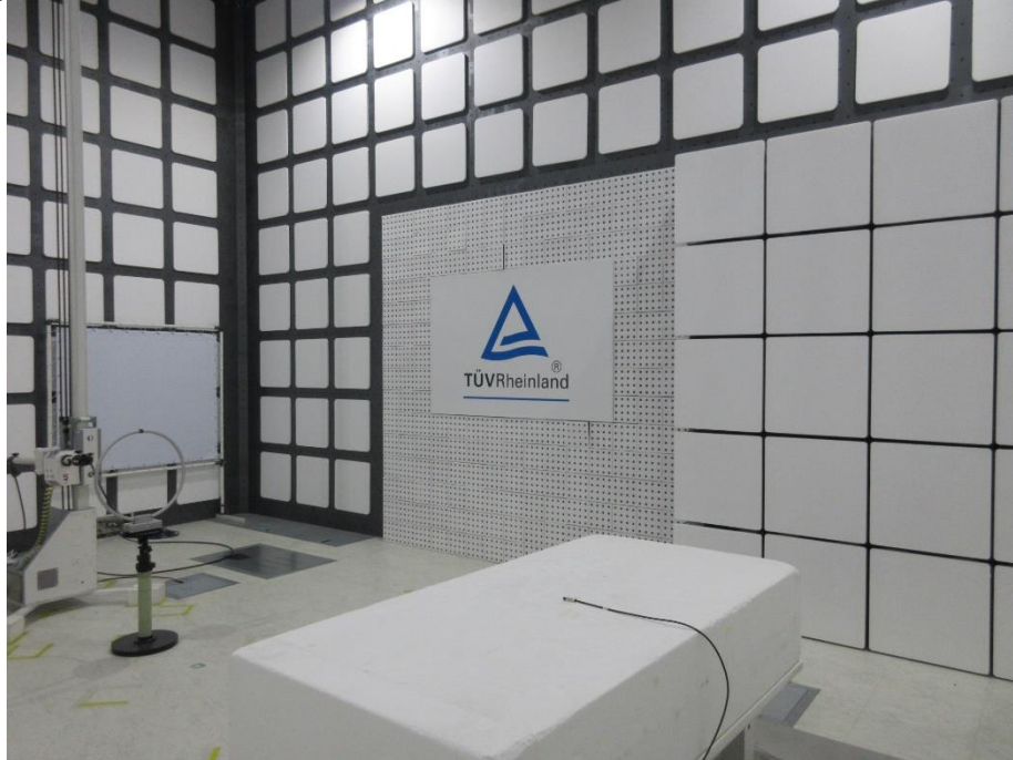
Photograph 3: Test Setup for Spurious Emissions (Back View 1)
