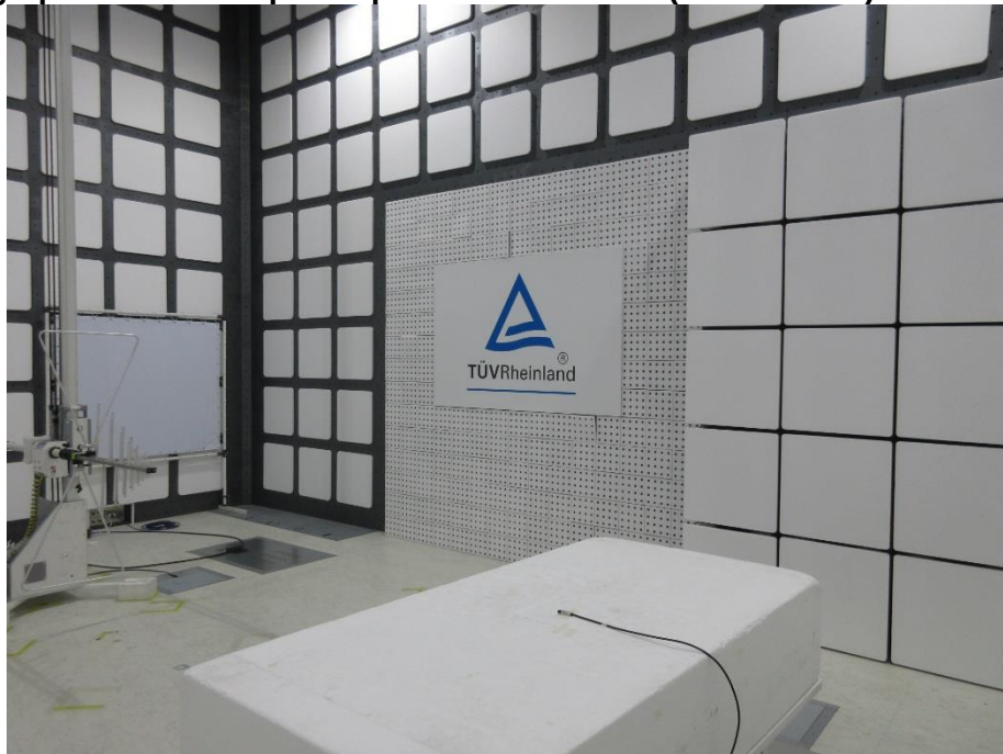
Photograph 4: Test Setup for Spurious Emissions (Back View 2)
