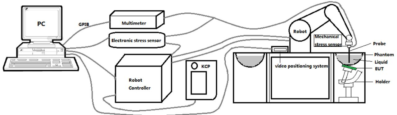
These measurements were performed with the automated near-field scanning system OPENSAR from SATIMO. The system is based on a high precision robot (working range: 901 mm), which positions the probes with a positional repeatability of better than  $\pm 0.03$  mm. The SAR measurements were conducted with dosimetric probe (manufactured by SATIMO), designed in the classical triangular configuration and optimized for dosimetric evaluation.
