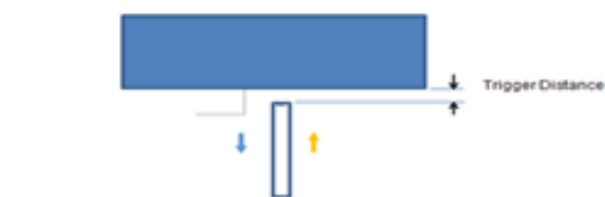
Picture proximity sensor triggering distance assessment top side
