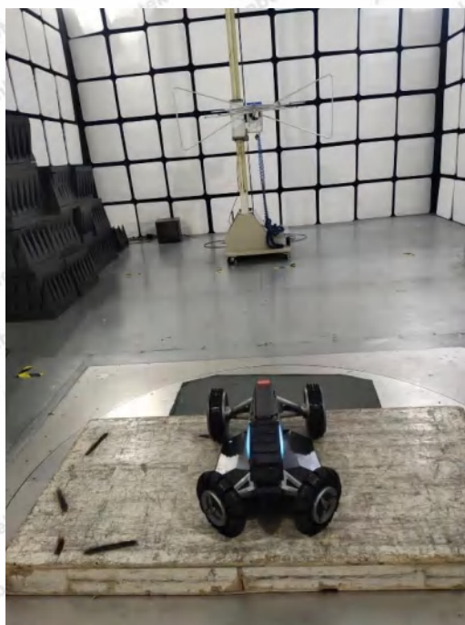
Photo of Radiation Spurious Emission Test
