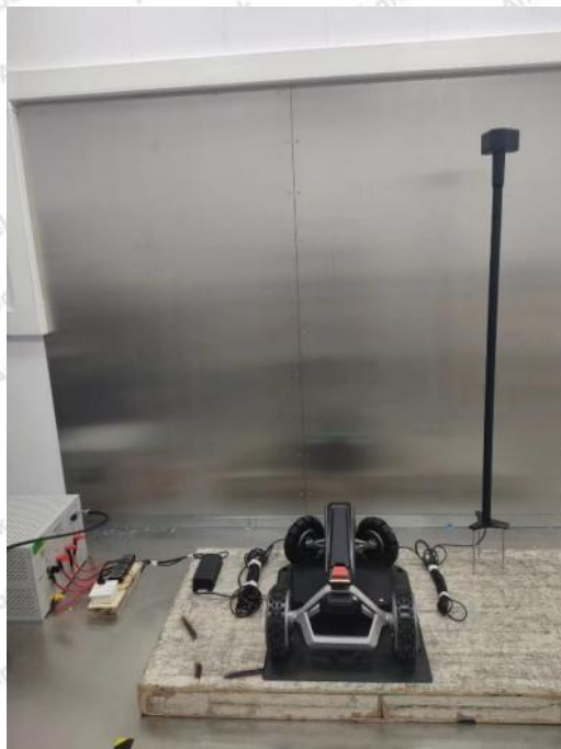
Photo of Conducted Emission Measurement
