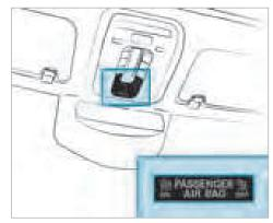
Vehicles without automatic front passenger airbag shutoff have a special sticker affixed to the side of the cockpit on the front passenger side  $(\rightarrow page 69)$ .
