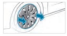
To remove: using both hands, carefully reach into two wheel trim openings and remove the wheel trim.
