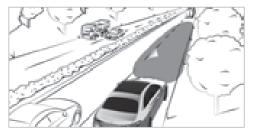
At speeds of at least 30 km/h, a triangle that indicates a lane correction and its direction will be projected onto the road in the following cases:
