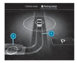
When the vehicle is stationary, indicated vehicle path (a) into currently selected parking space (s) also appears.
