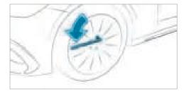
Using the wheel wrench, loosen the wheel bolts on the wheel you wish to change by about one full turn. Do not unscrew the screws completely.
