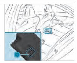
To lock or unlock: slide catch 1 upwards or downwards.
