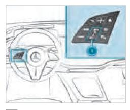
Adopts the stored/detected speed Deactivates Active Distance Assist DISTRONIC / the variable limiter
