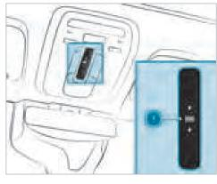
The sliding sunroof and the roller sunblind are operated using control panel 1.
