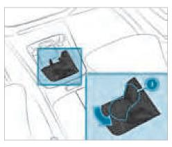
Push the side panel back in the direction of the arrow until it engages in correct position
