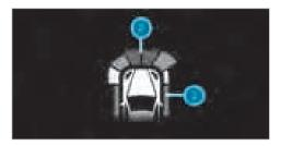
Optionally, obstacles detected by Parking Assist PARKTRONIC from a distance of approximately 1.0 m in front 2 and 0.7 m on sides 3 can also be displayed in the head-up display.
