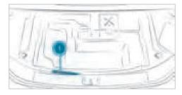
The towing eye  $\bigcirc$  is located under the boot floor in the loading sill.
