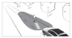
The spotlight function runs in the background and flashes the headlamps in four short bursts at persons detected within the lane markings. You will also be made aware of the position of the person by a projected symbol.
