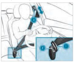
Always engage seat belt tongue 1 of the seat belt into seat belt buckle 2 of the corresponding seat.
