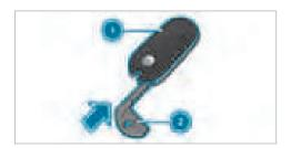
Press emergency key (2) into the opening in the key in the direction of the arrow until cover (1) opens. When doing so, do not hold cover (1) closed.
