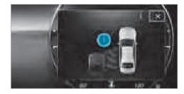
If a course-correcting brake application occurs, the red warning lamp flashes in the outside mirror and a warning tone sounds. In addition, a display (1) indicating the danger of a side collision
