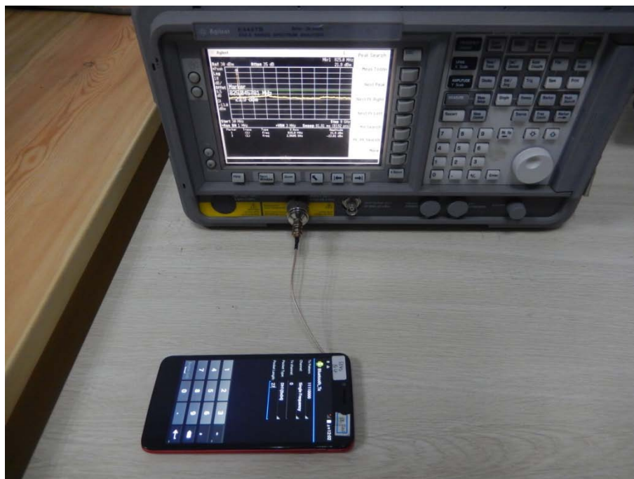
DSS&DTS RF conduction test photos
