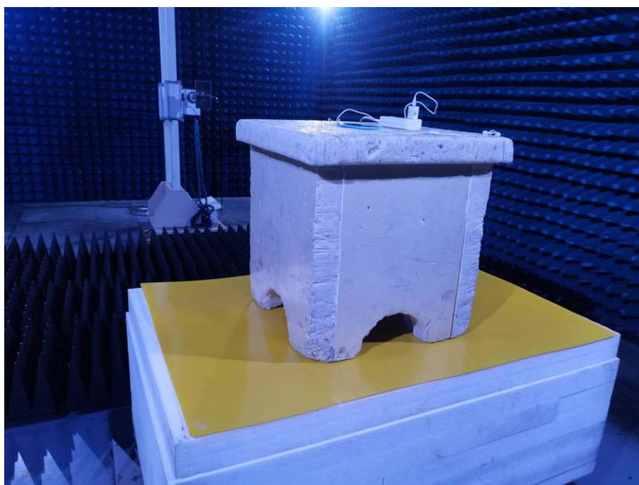
Photo of Radiated Emission Measurement (Above 1G)
