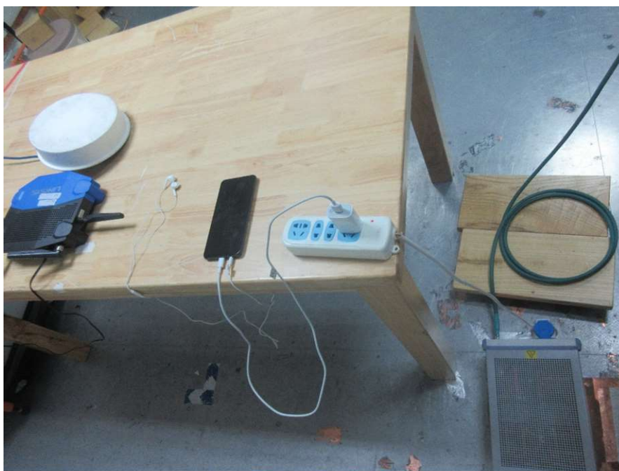
Conducted Emission 150kHz-30MHz (Rear view) – Mode 2
