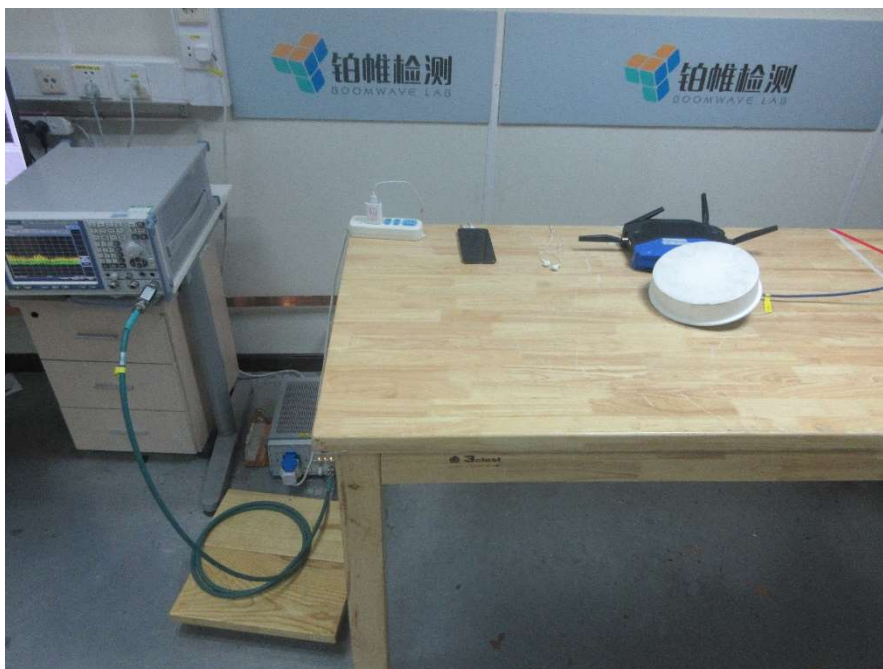
Conducted Emission 150kHz-30MHz (Front view) – Mode 2
