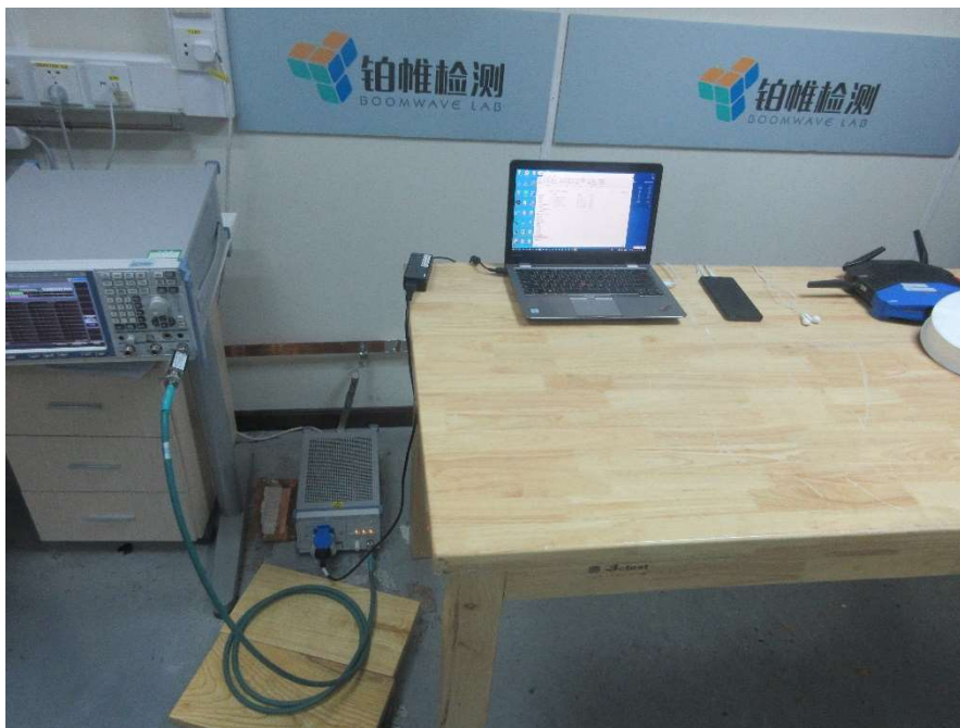
Conducted Emission 150kHz-30MHz (Front view) – Mode 5
