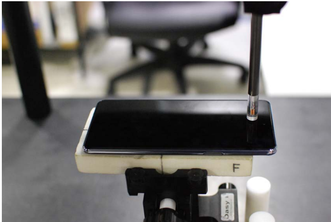
Figure 16-1 Test Setup for Wireless Device
