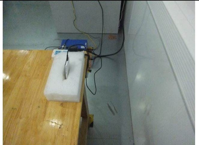
Conducted Emissions Test Setup Side View
