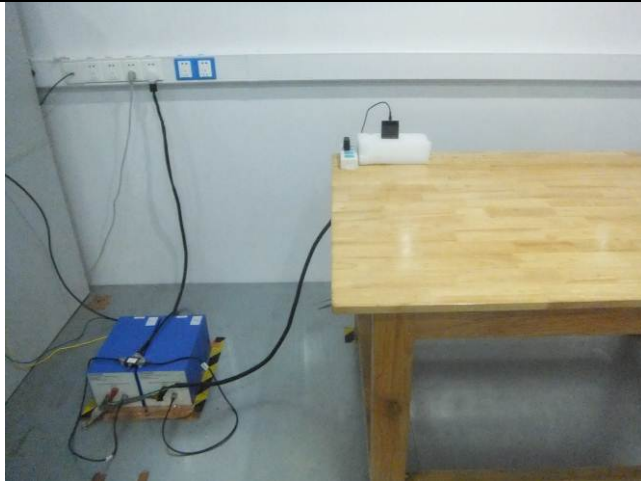
Conducted Emissions Test Setup Front View
