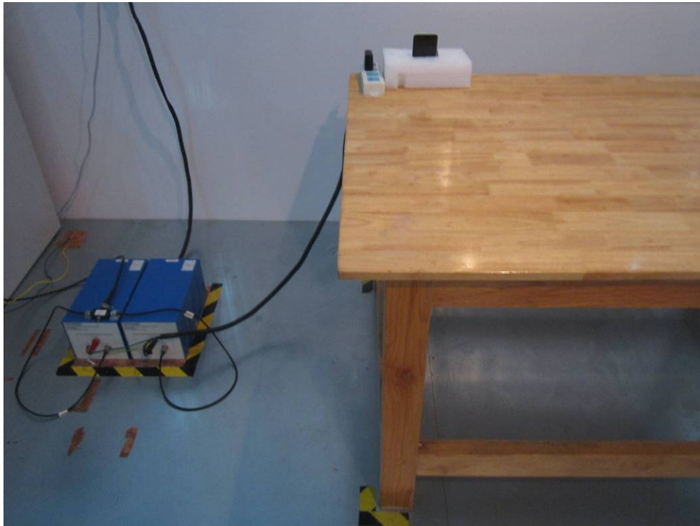
Conducted Emissions Test Setup Front View
