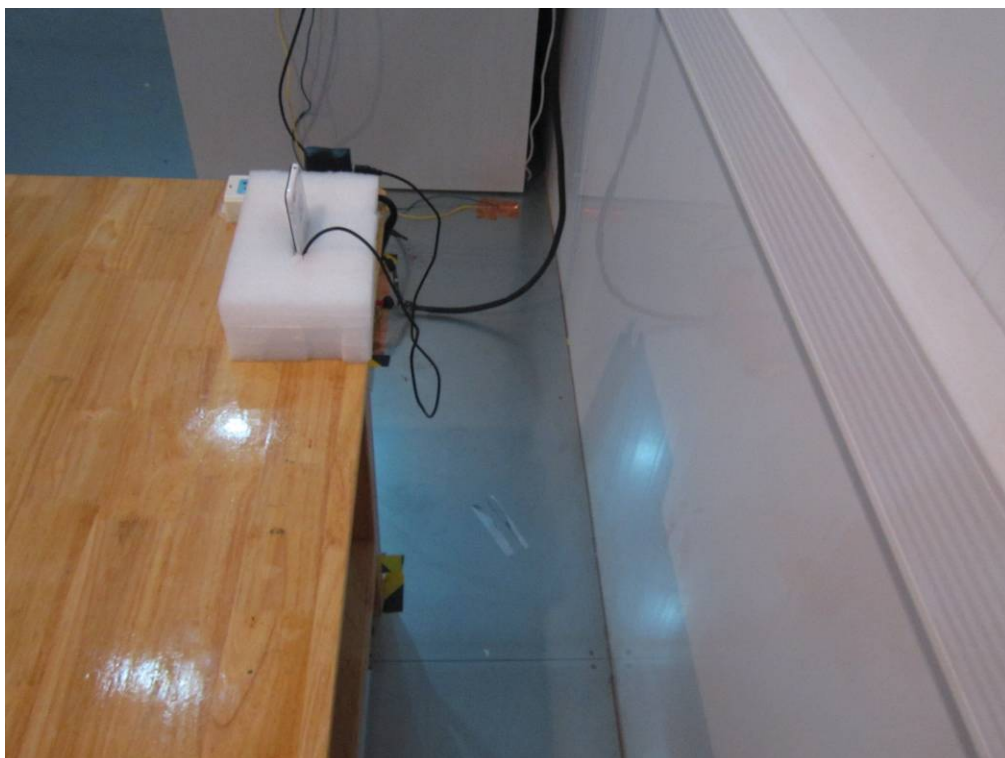
Conducted Emissions Test Setup Side View
