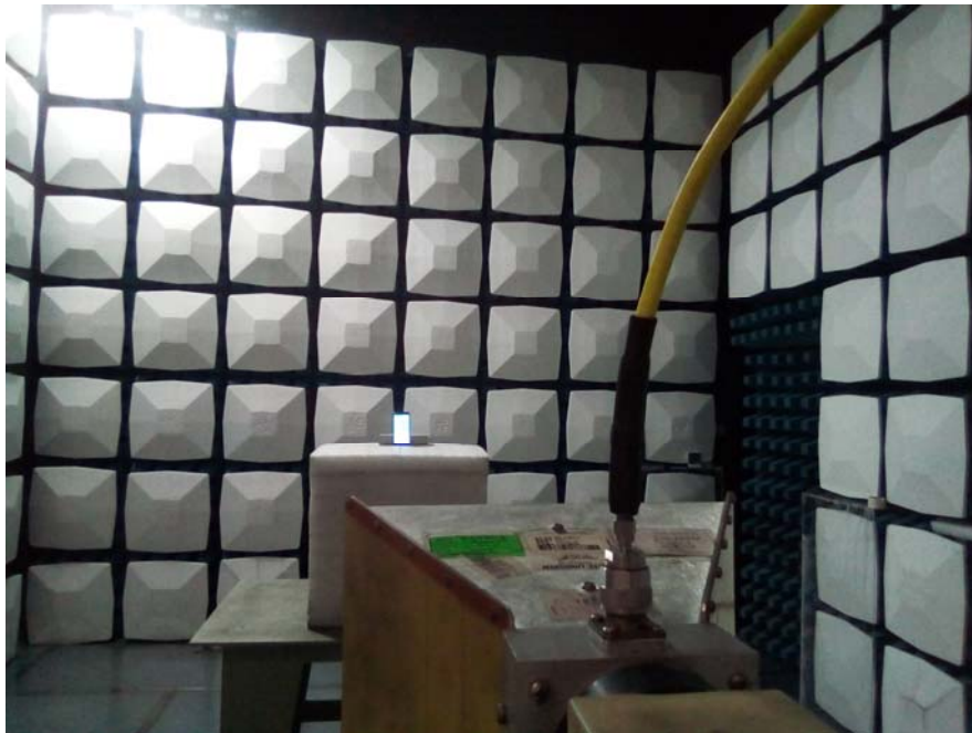
Radiated Emission Above 1GHz View
