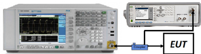
Figure 7-2. Test Instrument & Measurement Setup
