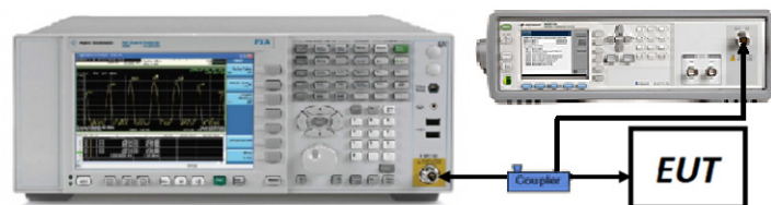
Figure 7-3. Test Instrument & Measurement Setup
