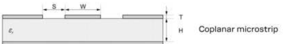
Figure 26: Coplanar micro-strip dimension specification
