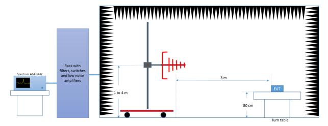
Radiated Setup 1 GHz - 18 GHz
