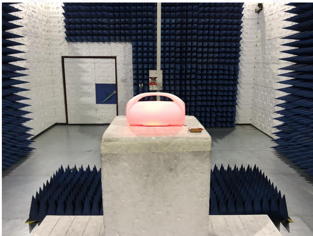
RADIATED EMISSION TEST SETUP ABOVE 1GHZ
