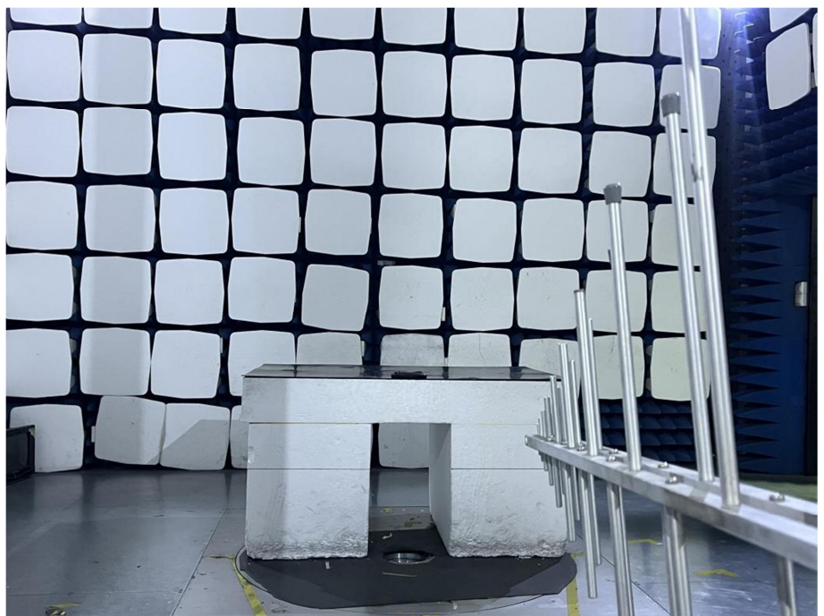
Radiation Emission Test Setup (30MHz to 1GHz)
