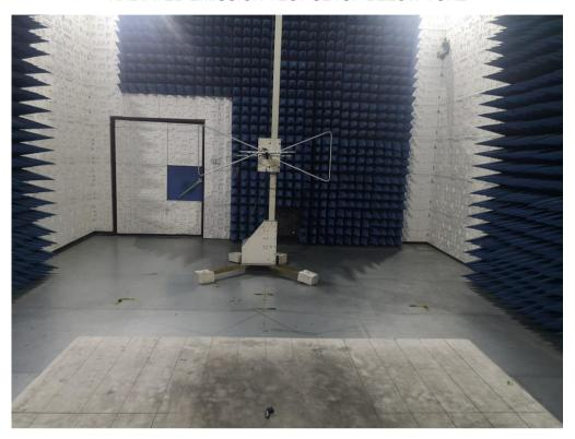
RADIATED EMISSION TEST SETUP ABOVE 1GHZ
