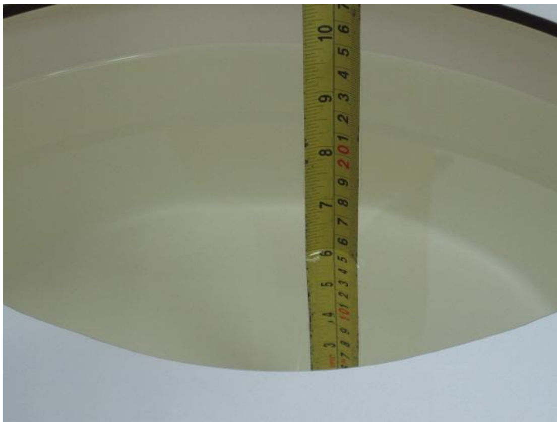
Picture C.3: Liquid depth in the flat Phantom (1900 MHz) (15.2cm deep)
