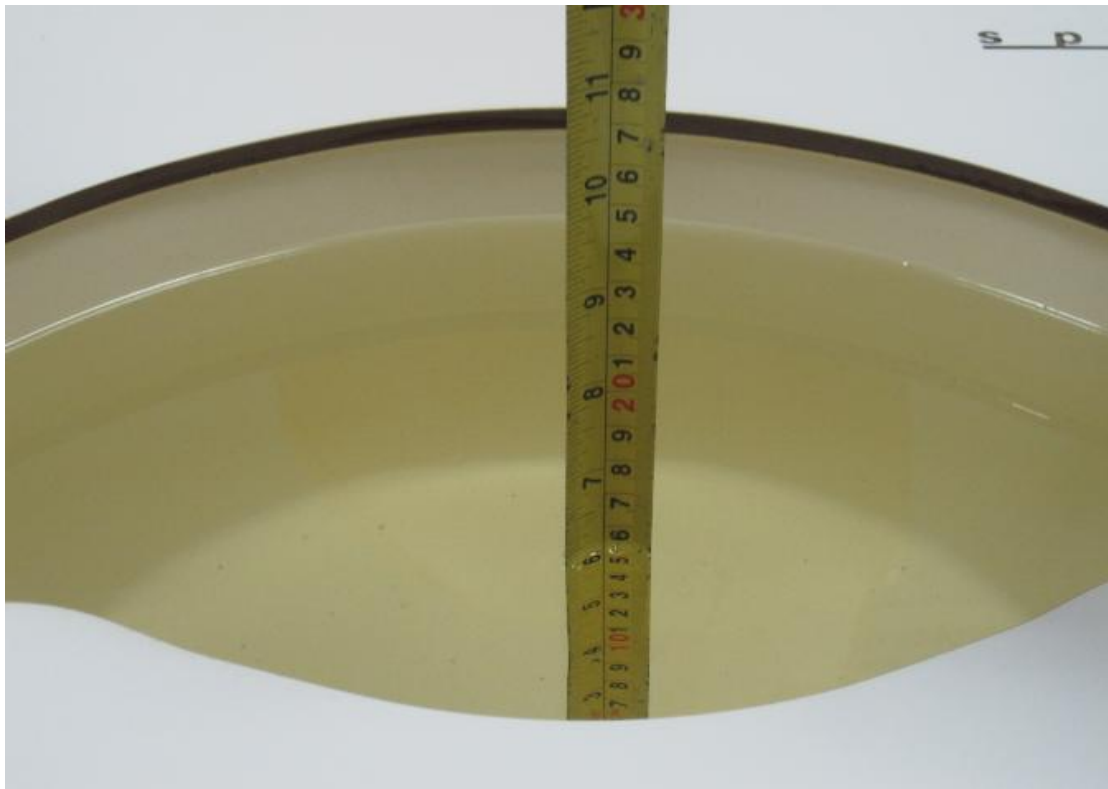
Picture C.2: Liquid depth in the flat Phantom (835MHz) (15.3cm deep)
