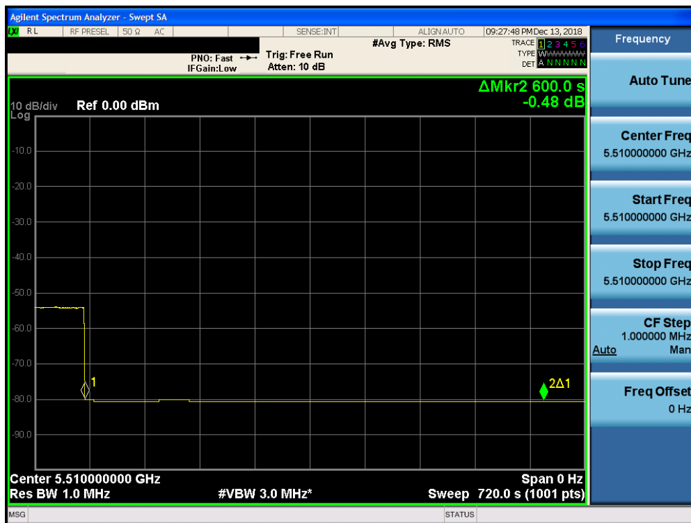
Figure 5-6. Band 2C Client Beacon Test – Monitoring live spectrum – Elapse time 10 minutes
