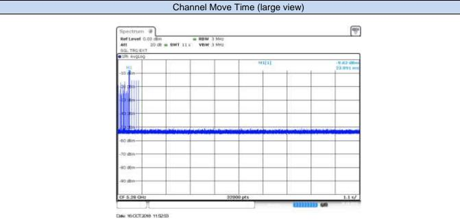
Marker M1 shows the end of the radar signal. Channel move time < 10s. Test PASS
