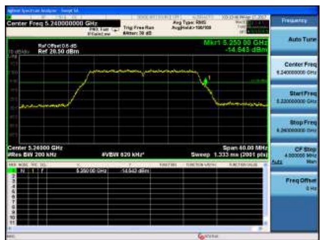
802.11ac-VHT80 - Channel 42 (5210MHz)
