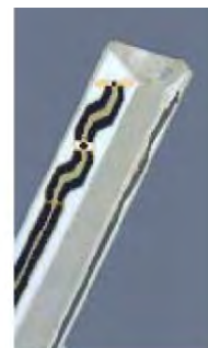
Figure F.2.2 Probe Thick-Film Technique
