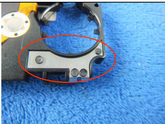
WIFI - Antenna View
