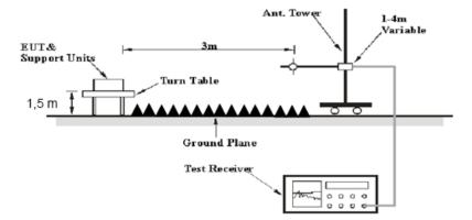
The radiated emissions were performed in the 3 meters distance, using the setup accordance with the ANSI C63.10-2013. The specification used was the FCC 15.209, FCC 15.247, RSS-247 and RSS-Gen limits.
