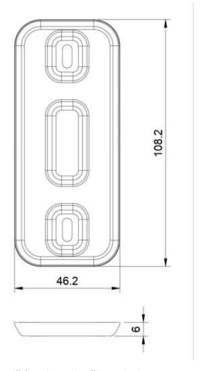
All dimensions are in millimeters (mm).
