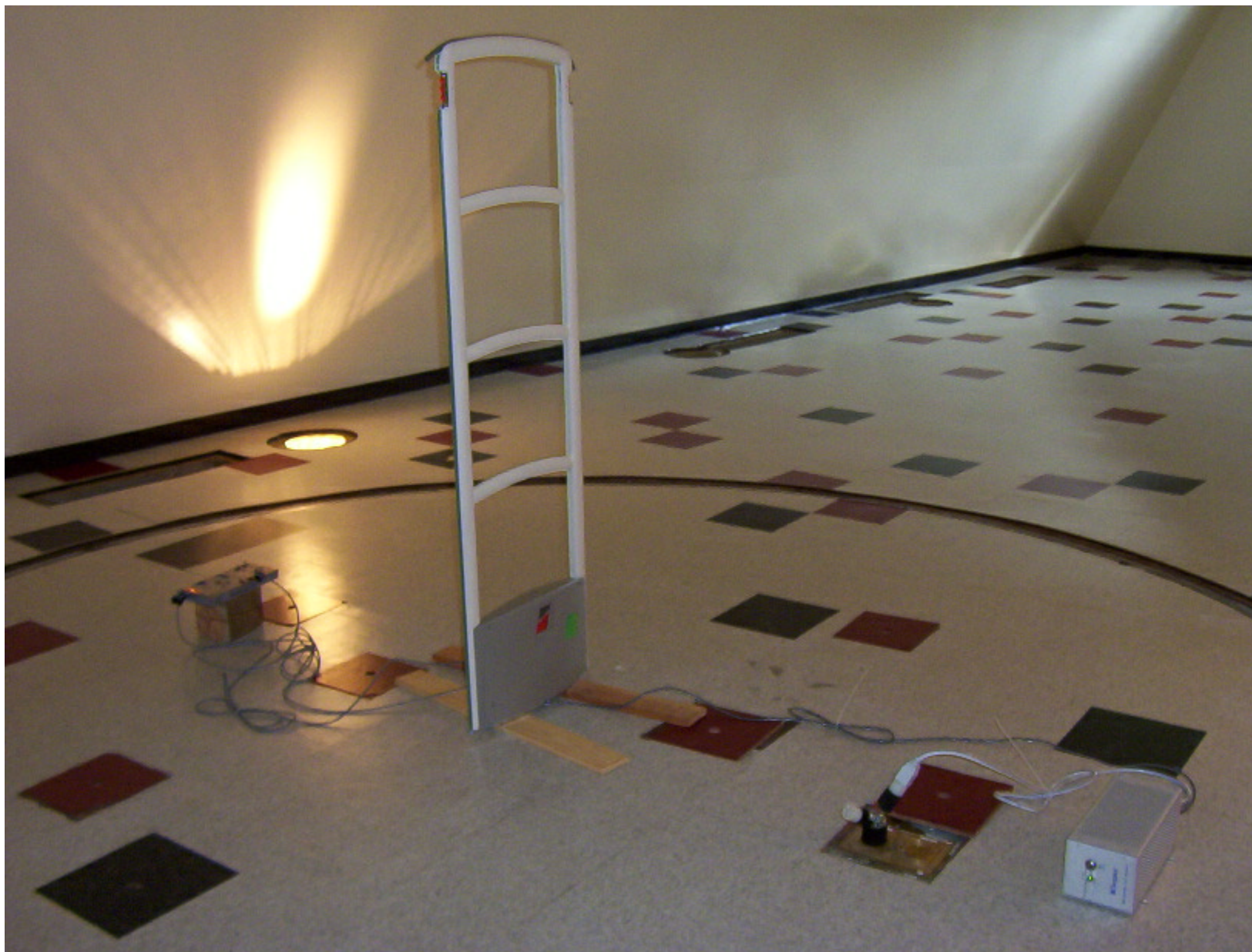
PHOTO 3 – LIBERTY DX SIDE VIEW OF RADIATED EMISSIONS TEST SETUP
