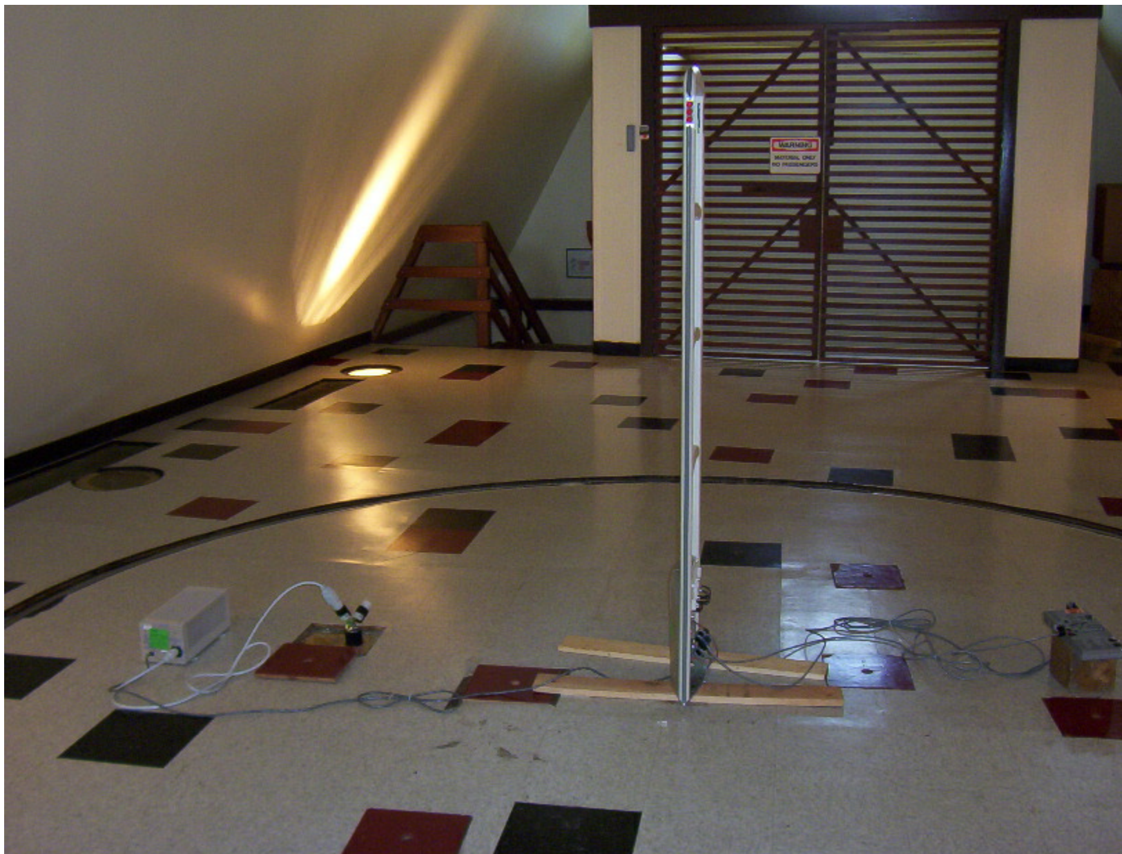
PHOTO 2 – LIBERTY DX REAR VIEW OF RADIATED EMISSIONS TEST SETUP
