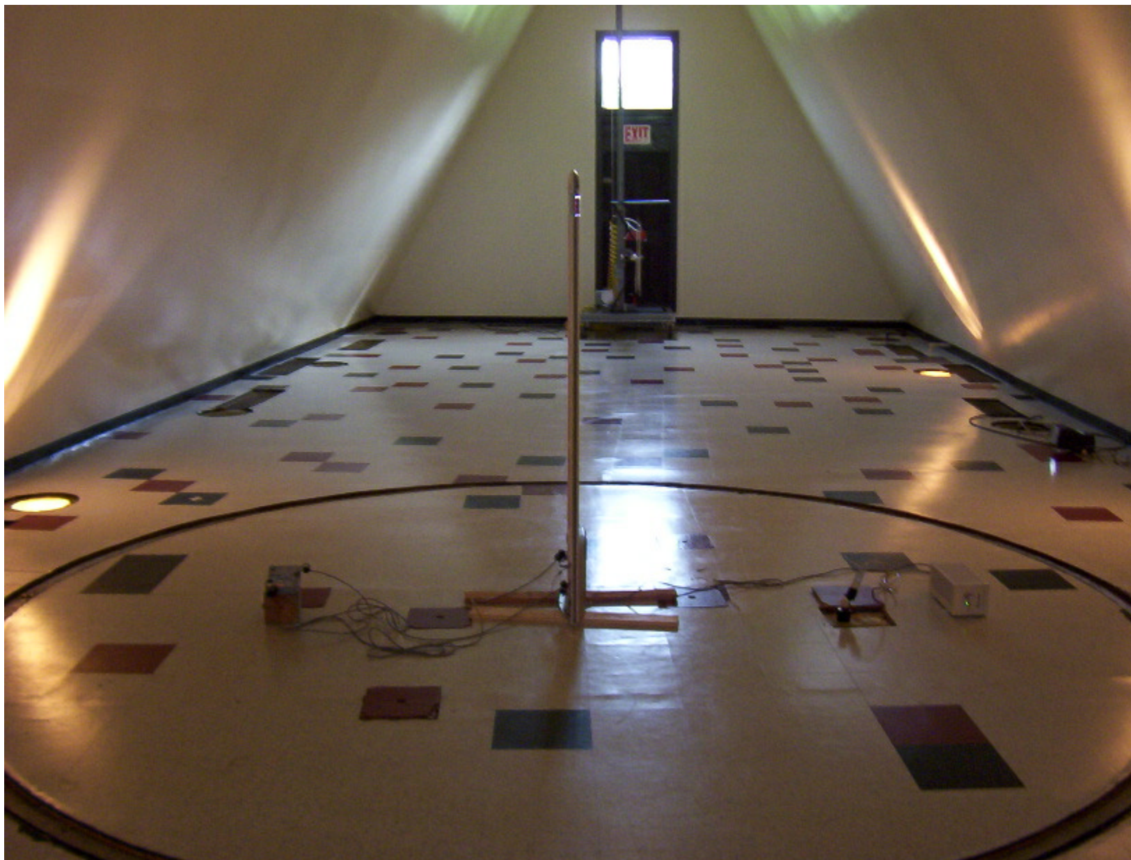
PHOTO 1 – LIBERTY DX FRONT VIEW OF TEST SETUP FOR RADIATED EMISSIONS
