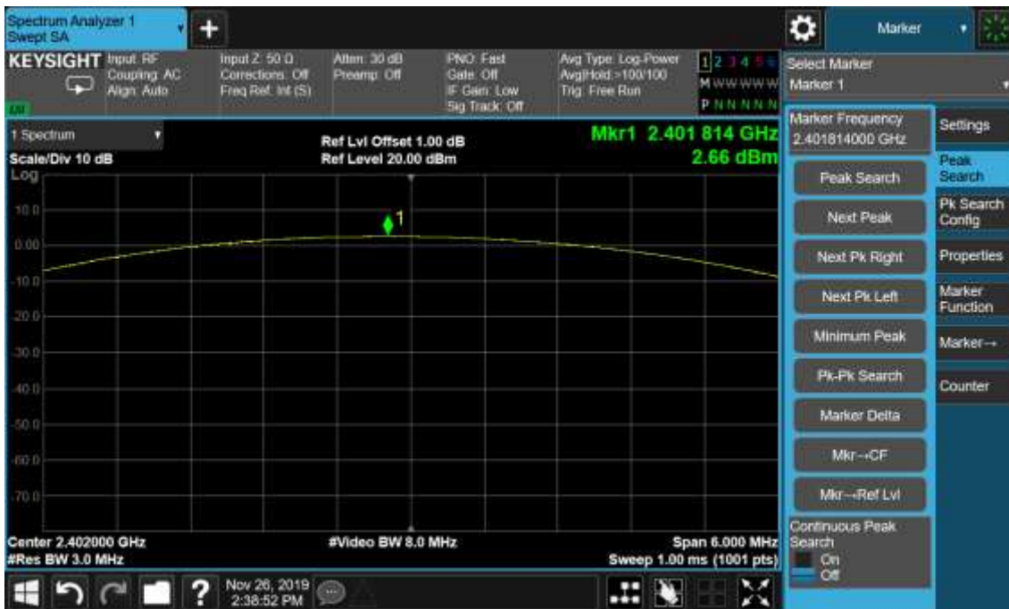
Figure 4: Maximum Conducted Output Power, 2402MHz, \pi/4 -QPSK
