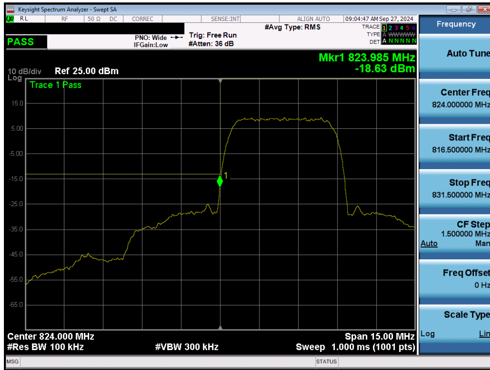
Plot 7-78. Lower Band Edge Plot (WCDMA Cell – Ch. 4132 – Ant1)
