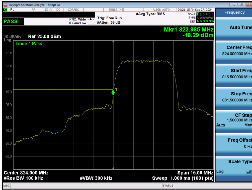
Plot 7-86. Lower Band Edge Plot (WCDMA Cell – Ch. 4132 – Ant2)
