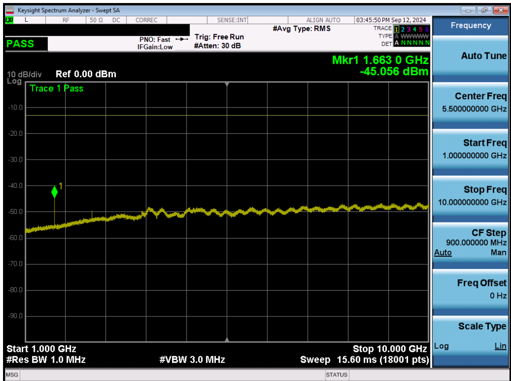
Plot 7-72. Conducted Spurious Plot (LTE Band 26/5 - 10MHz QPSK - 1 RB - Low Channel – Ant2)
