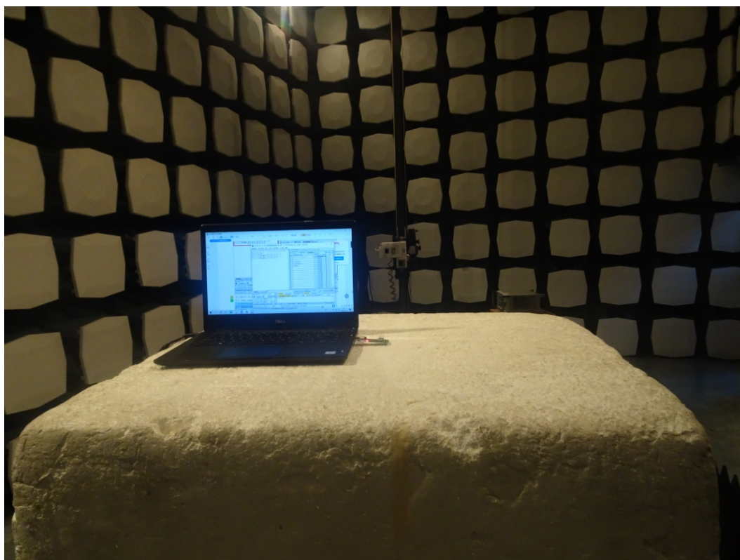
Picture 1 Radiated Emission Test Setup
