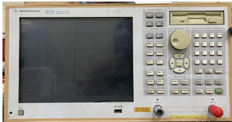
Agilent 5071B (S Parameter (RL/VSWR) Test Equipment)
