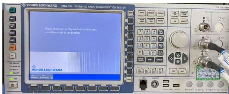
CMW 500 (2G/3G/4G Test Equipment)
