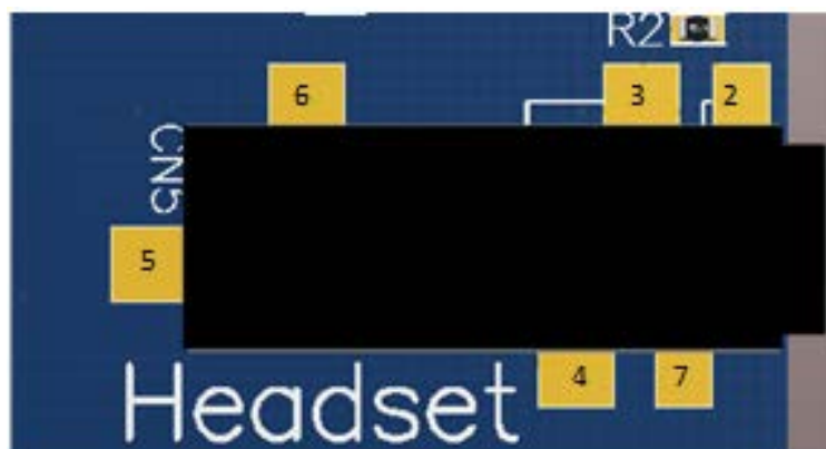
Figure 12. Audio jack connector MB1262/CN5
