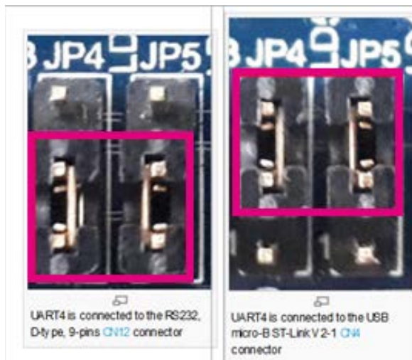
Figure 18. HW configuration for the RS-232 interface
