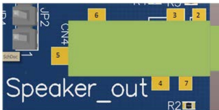
Figure 13. Audio jack connector MB1262/CN4
