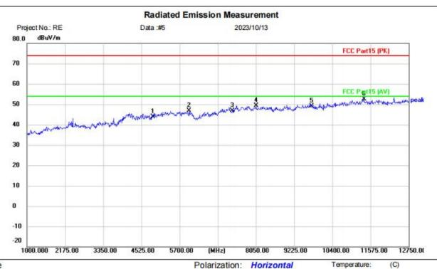
Site Polarization: Horizontal Temperature: (C Limit: FCC Part15 (PK) Power: Humidity: %RH
