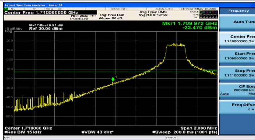
Channel Bandwidth: 10 MHz_LCH_QPSK_1RB#24
