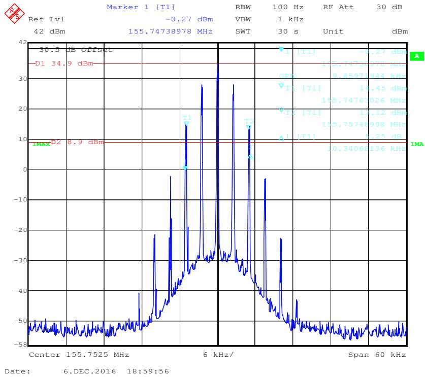
**Frequency 155.7525 MHz: 99% Occupied & 26 dB Bandwidth, Low Power**
