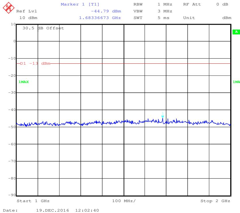
**30MHz – 1 GHz, Spacing Channel 12.5 kHz, 155.7525 MHz**
