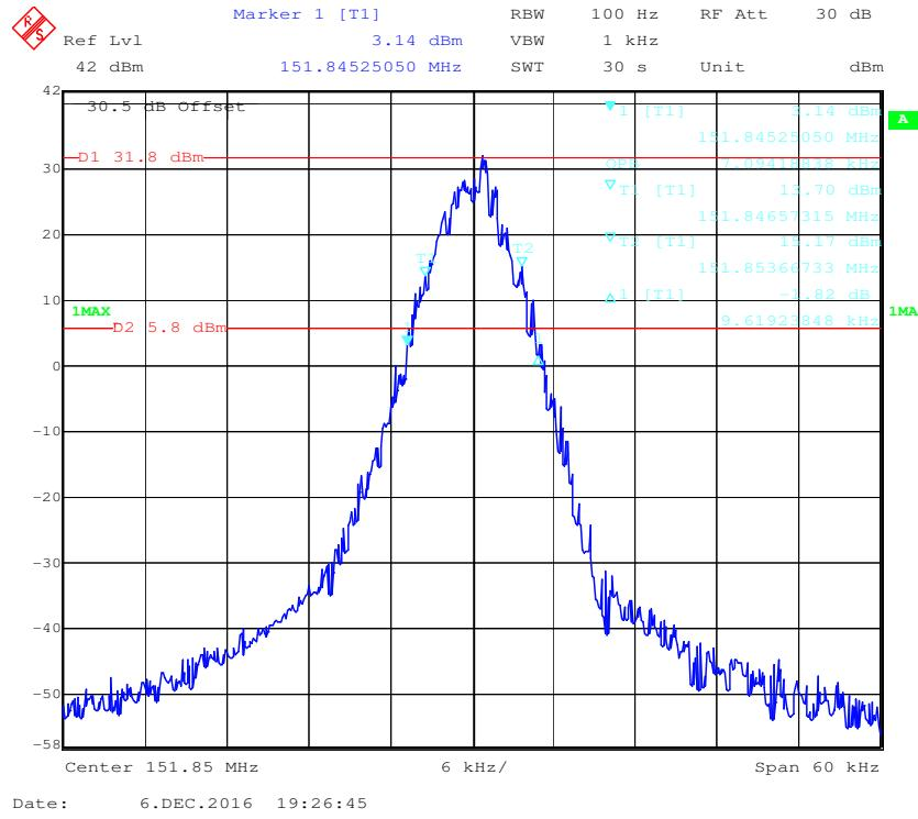
**Frequency 151.85 MHz: 99% Occupied & 26 dB Bandwidth with Low Power**
