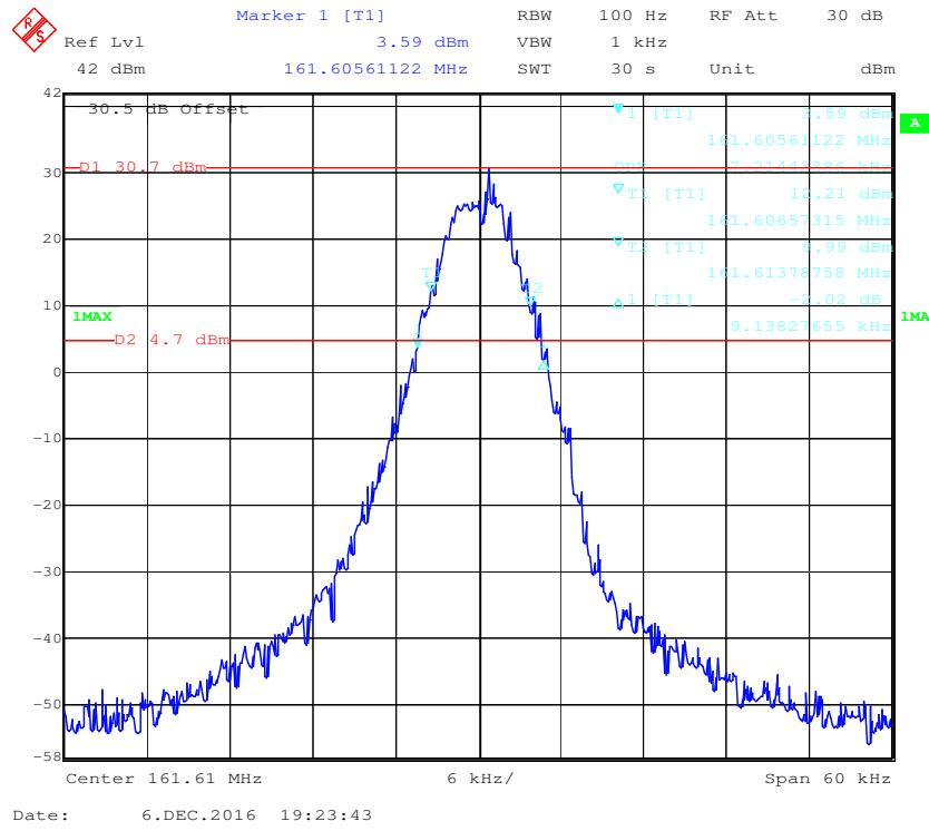
**Frequency 161.61 MHz: 99% Occupied & 26 dB Bandwidth with Low Power**
