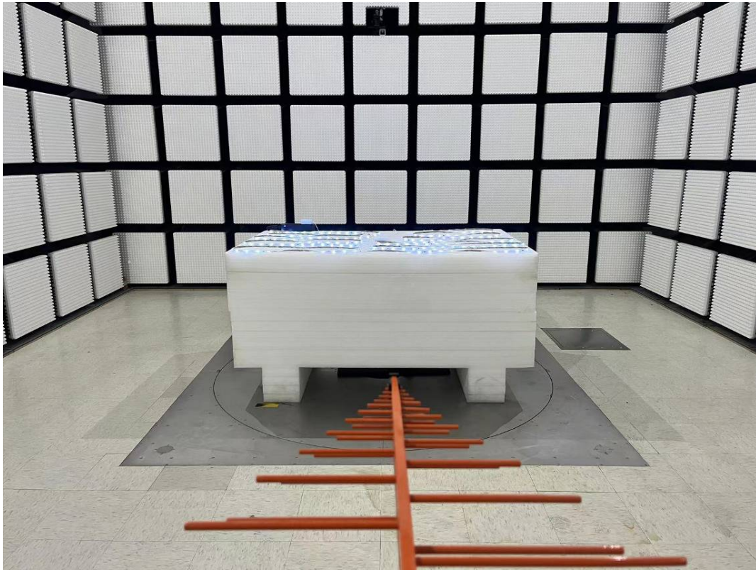
Radiated Emission Above 1GHz View(For model MLW7-1003-ICM)
