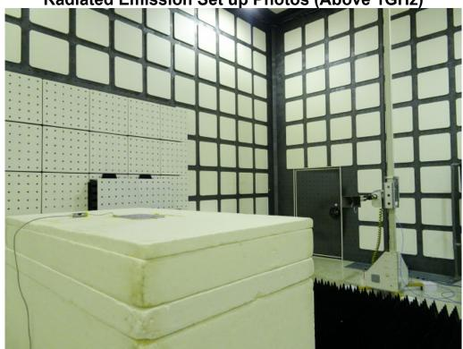
Radiated Emission Set up Photos (Front View)
