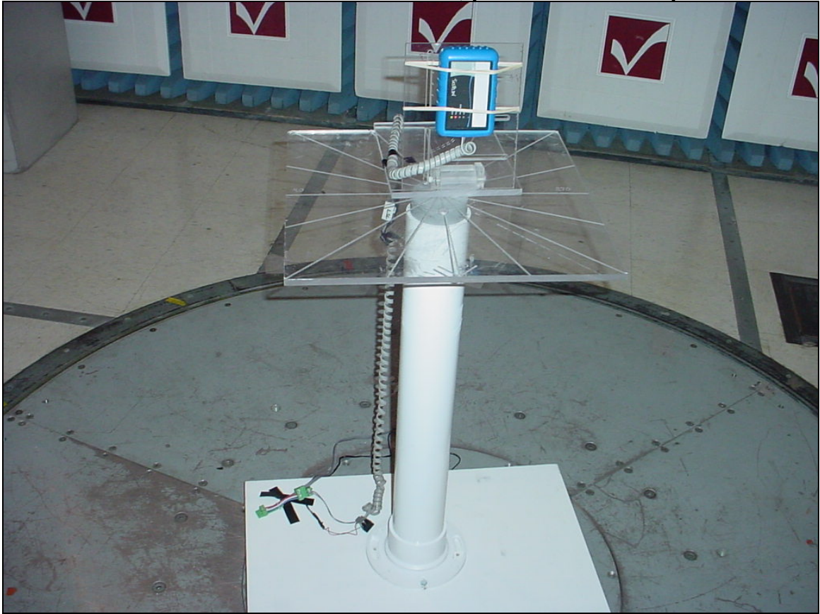
View of the EUT in vertical orientation, placed on the test pedestal.
